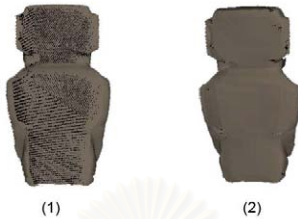
Figure 3-7: Hit range threshold. (1) Hit range threshold e = 0.01 . (2) Hit range threshold e = 0.02 .
