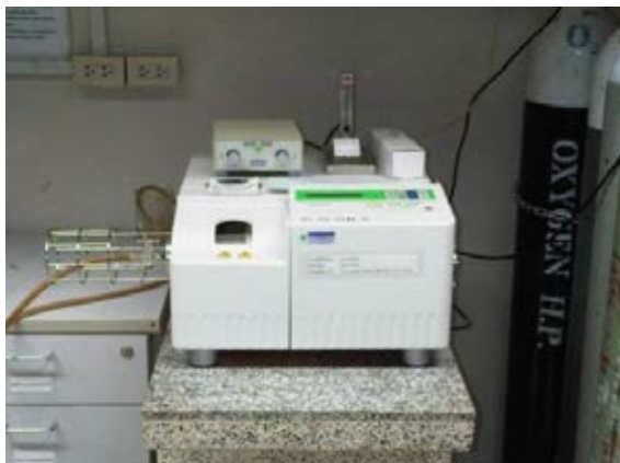
Figure 3.6 Thermogravimetric Analyzer, Mettler Toledo TGA/SDTA 851 e
