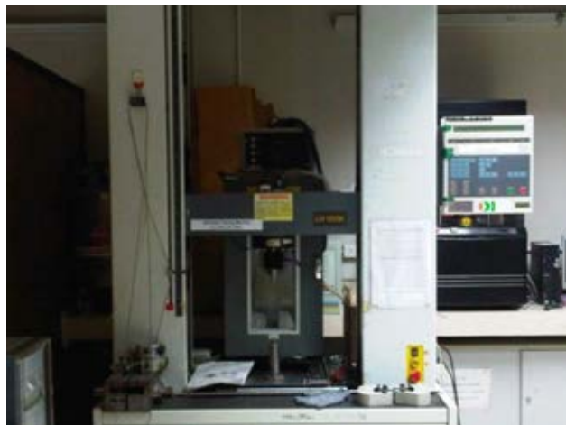
Figure 3.11 Universal Testing Machine, LLOYD LR 100K
