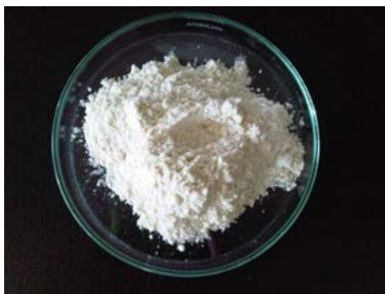
Figure 4.1 Physical appearance of acid hydrolyzed CT-MCC
