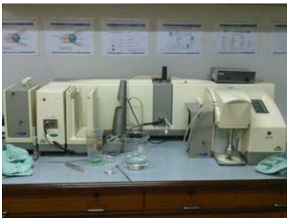
Figure 3.4 Laser Particle Size Analyzer, Malvern Instruments Mastersizer 2000
