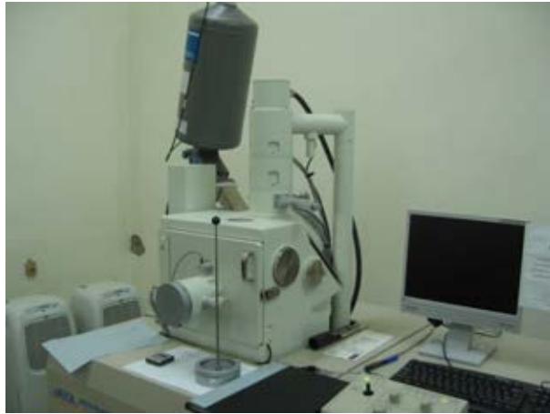
Figure 3.10 Scanning electron microscope, JEOL JSM-6480LV
