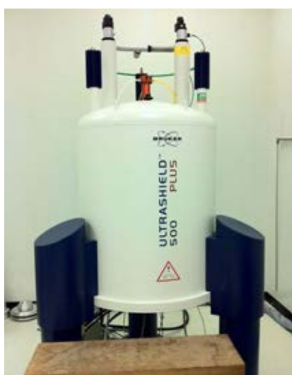
Figure 3.8 Carbon Nuclear Magnetic Resonance Spectroscopy, Bruker DPX-300 MHz NMR Spectrometer
