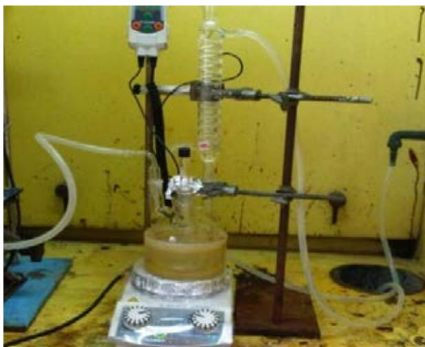
Figure 3.3 Experimental set up for PLA-g-MA solution polymerization.
