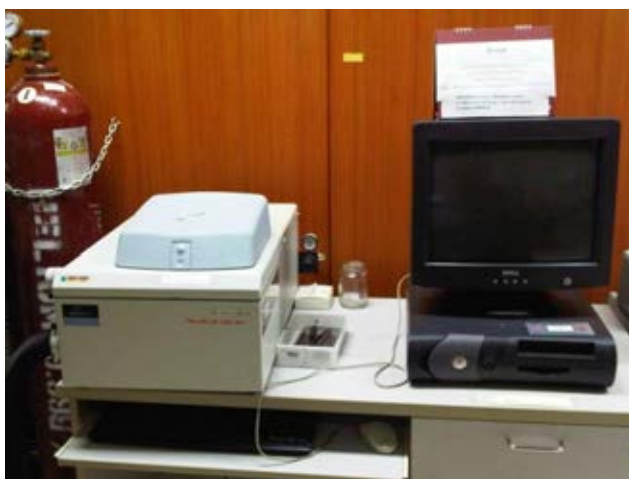
Figure 3.9 Differential Scanning Calorimeter, PerkinElmer Pyris Diamond DSC
