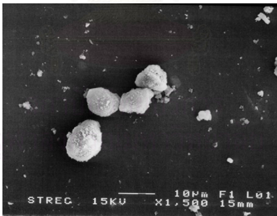
Figure 5.9 Scanning electron micrograph of Ga/MFI (6.0 μm) catalyst.
