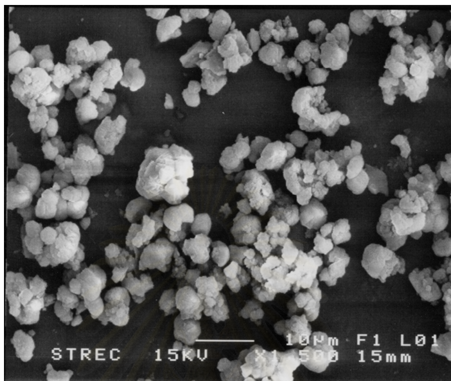
Figure 5.8 Scanning electron micrograph of Ga/MFI (4.1 μm) catalyst.
