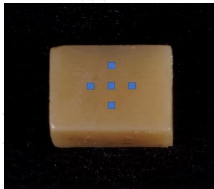
Figure 10 Position for measured Ra of the specimen
