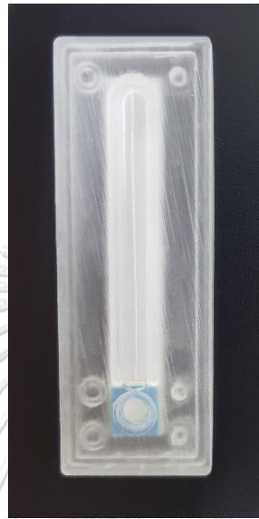
Figure 4.23 A new platform of 3D printed device holder coupled with the cotton thread-based device.
