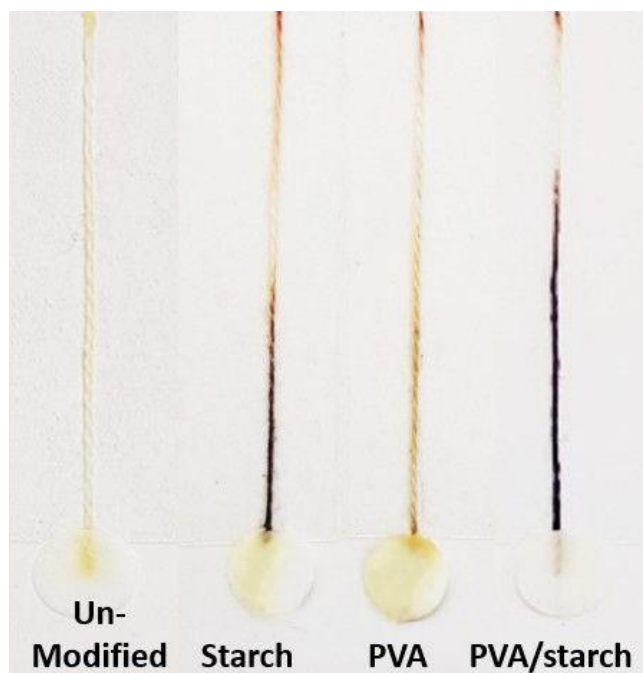
Figure 4.1 Color change of the different modifications of the cotton thread after the measurement of 5 mM H_2O_2 .
