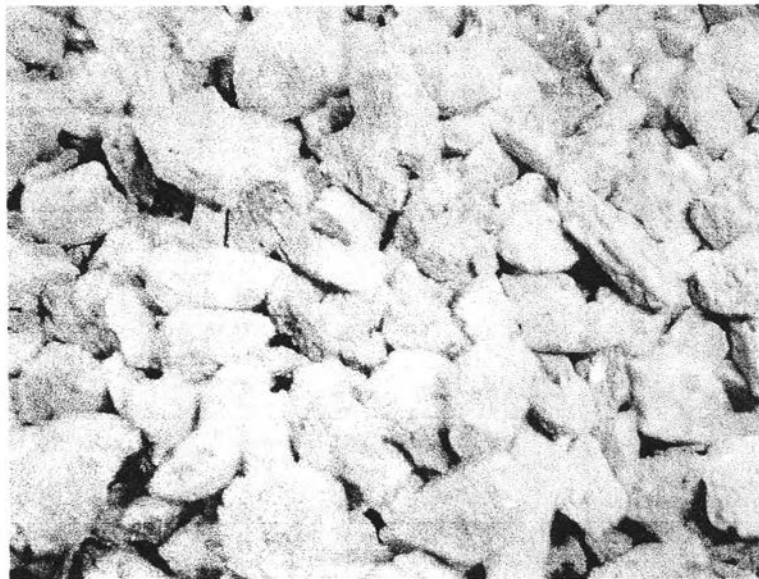
Figure 3.3 4.0-4.75 mm pumice with the US standard sieve.
