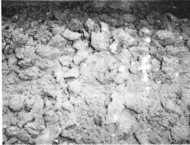
Figure 3.2 Grind pumice from coarse grinder.
