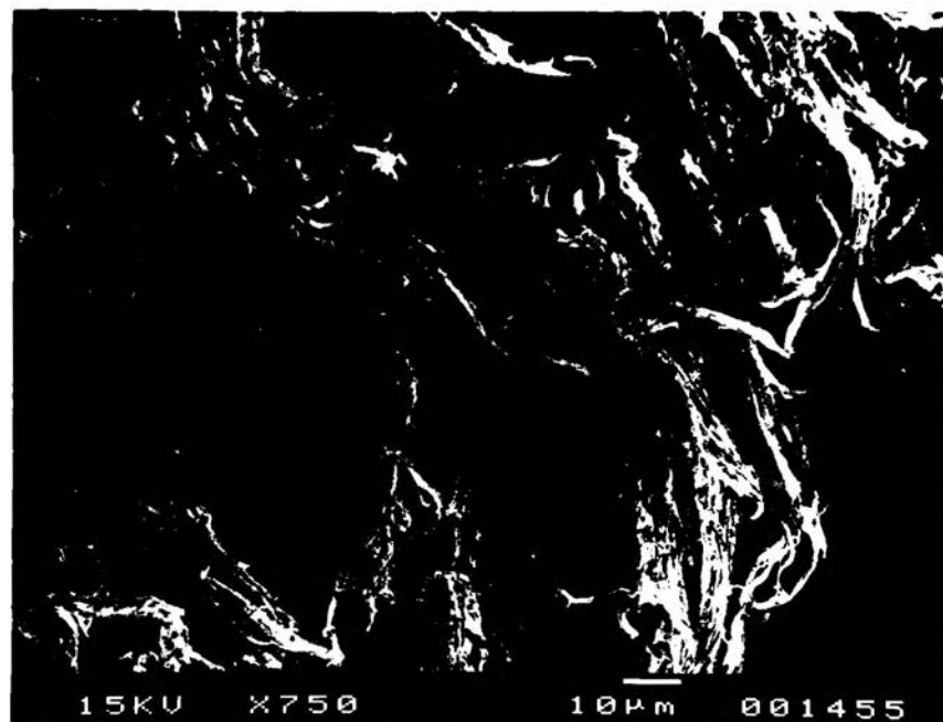
Figure 4.4.1 Scanning electron micrograph of fracture surface of tensile specimens for 0.20 calcined bone ash volume fraction.
