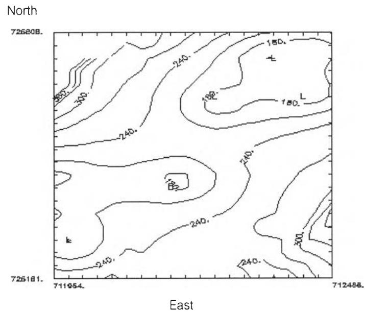
Fig. 5.11. The standard error of estimation computed for a kriged estimation of calorific value, S2 seam, Ban Khok Ok deposit, Saba Yoi area.
