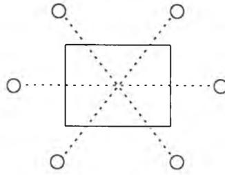
Fig. 5.1 Inverse distance method for geostatistical estimation
