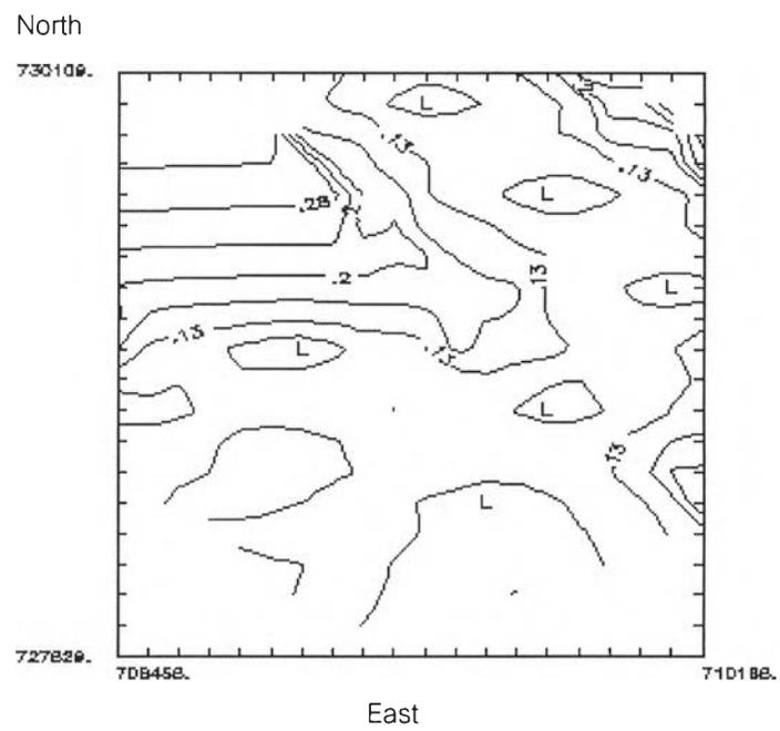
Fig. 5.19. Standard error of estimation for sulphur content (%), S3 seam, Ban Sao deposit, Saba Yoi area.
