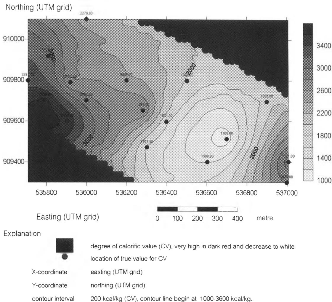
Fig. 5.8. Kriging estimate as shown by colour-shaded relief and contour lines for calorific value (kcal/kg), P2 seam, Nong Wa deposit, Sin Pun area.
