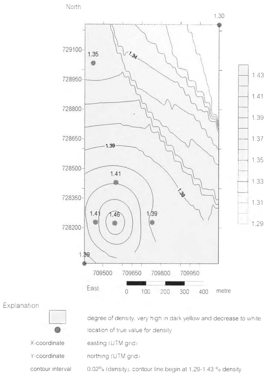
Fig. 5.22. Kriging estimation as shown by colour-shaded relief and contour lines for density (g/cc), S4 seam, Ban Sao deposit. Saba Yoi area.
