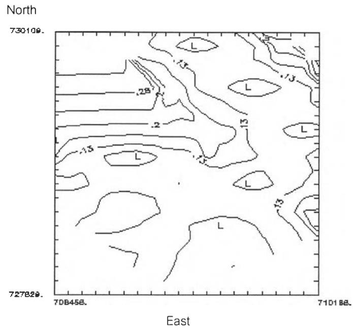
Fig. 5.15. Standard error of estimation for moisture content (%), S3 seam, Ban Sao deposit, Saba Yoi area.
