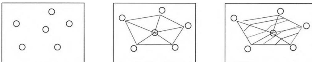
Triangulation method of estimating positions of contour lines
