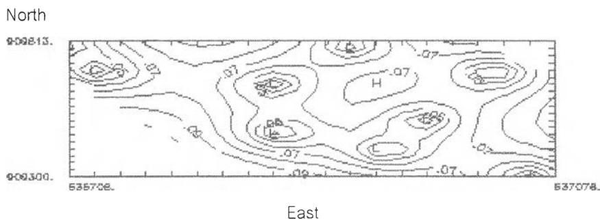
Fig. 5.21. Standard error of estimation for density (g/cc), M seam, Nong Wa deposit, Sin Pun area.
