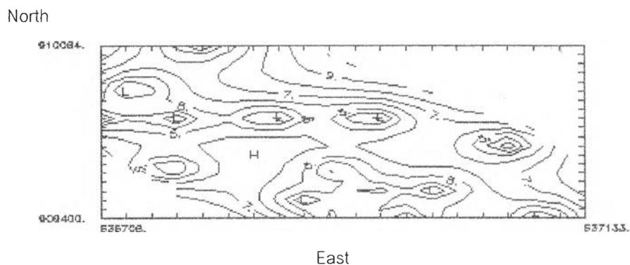
Fig. 5.5. Standard error of estimation for ash content (%), P1 seam, Nong Wa deposit, Sin Pun area.
