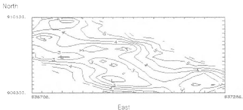
Fig. 5.13. Standard error of estimation for moisture content (%), P4 seam. Nong Wa deposit, Sin Pun area.
