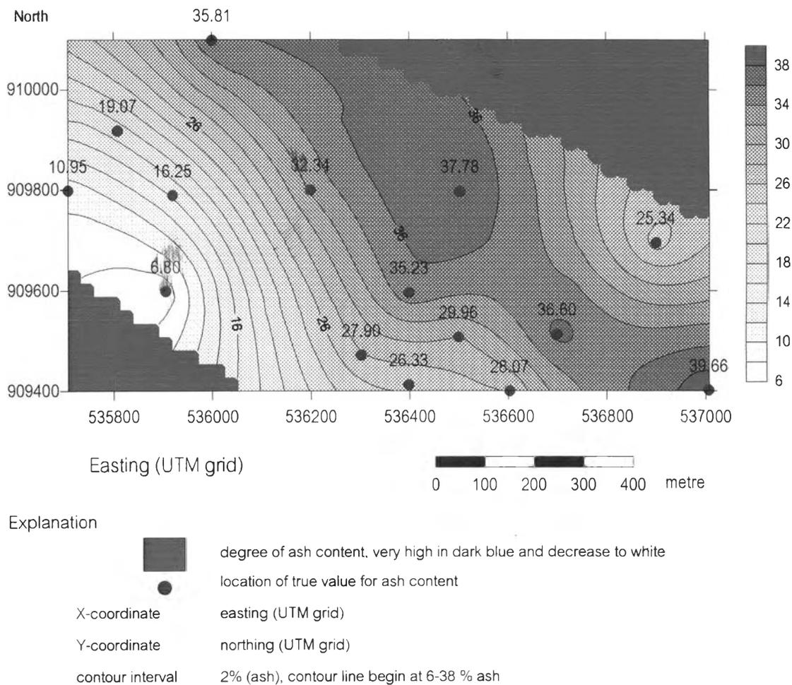
Fig. 5.4. Kriged estimate as shown by colour-shaded relief and contour lines for ash content (%), P1 seam, Nong Wa deposit, Sin Pun area.
