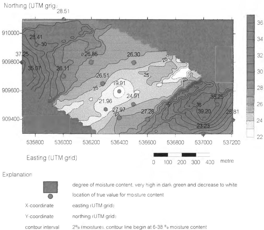
Fig. 5.12. Kriging estimate as shown by colour-shaded relief and contour lines for moisture content (%), P4 seam, Nong Wa deposit, Sin Pun area.
