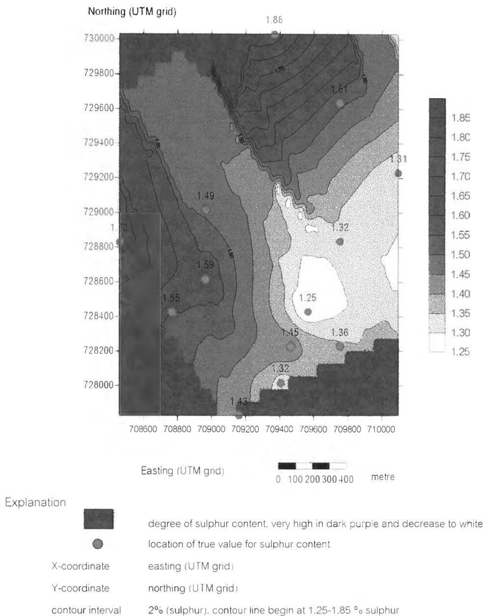
Fig. 5.18. Kriging estimate as shown by colour-shaded relief and contour lines for sulphur content (%), S3 seam, Ban Sao deposit, Saba Yoi area.
