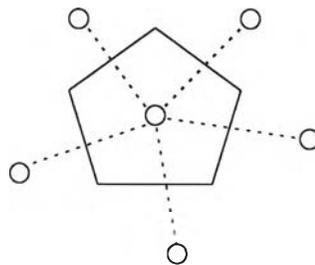
Fig. 5.2 Polygonal method for geostatistical estimation
