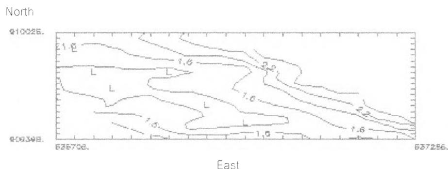
Fig. 5.17. Standard error of estimation for sulphur content (%), P3 seam, Nong Wa deposit, Sin Pun area.
