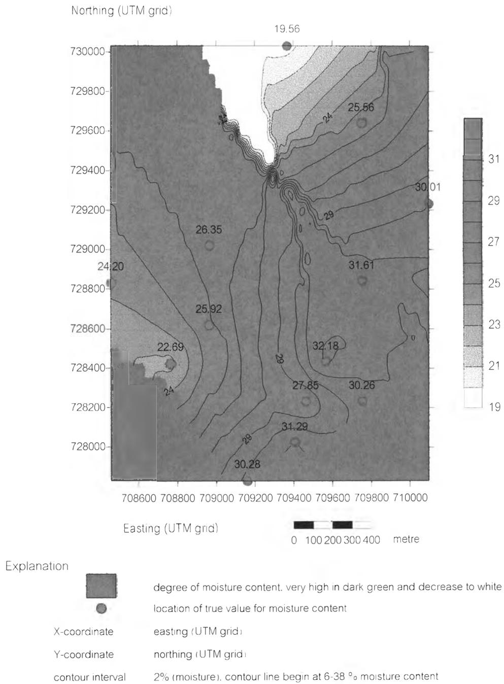
Fig. 5.14. Krigé estimate as shown by colour-shaded relief and contour lines for moisture content (%), S3 seam, Ban Sao deposit, Saba Yoi area.
