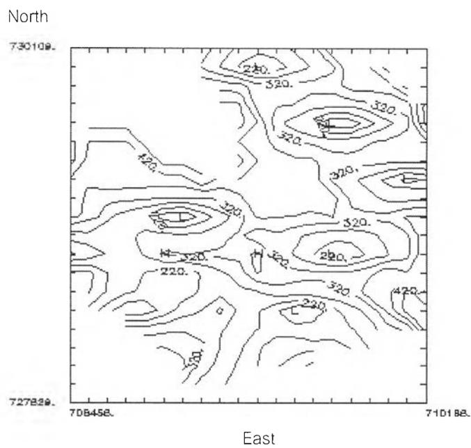
Fig. 5.7. Standard error of estimation for ash content (%), S3 seam, Ban Sao deposit, Saba Yoi area.
