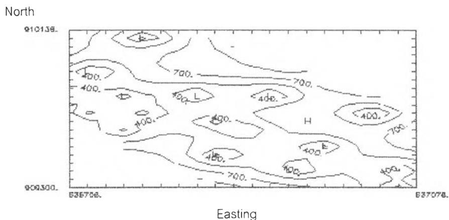
Fig. 5.9. The standard error of estimation computed for a kriged estimation of calorific value, P2 seam, Nong Wa deposit, Sin Pun area.
