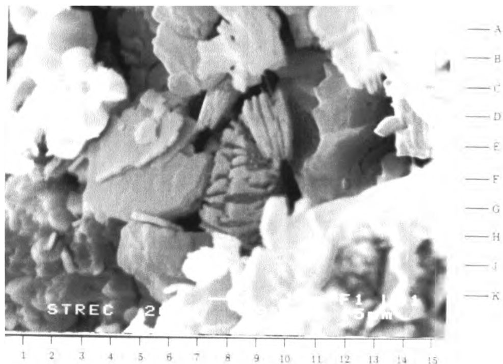
Fig. 3.30 Scanning electron micrograph of weathered rhyolitic tuff showing the mixtures of kaolinite (A7, J6) and illite (F7, F9) (see EDS curves in Figures 3.34 and 3.35).
