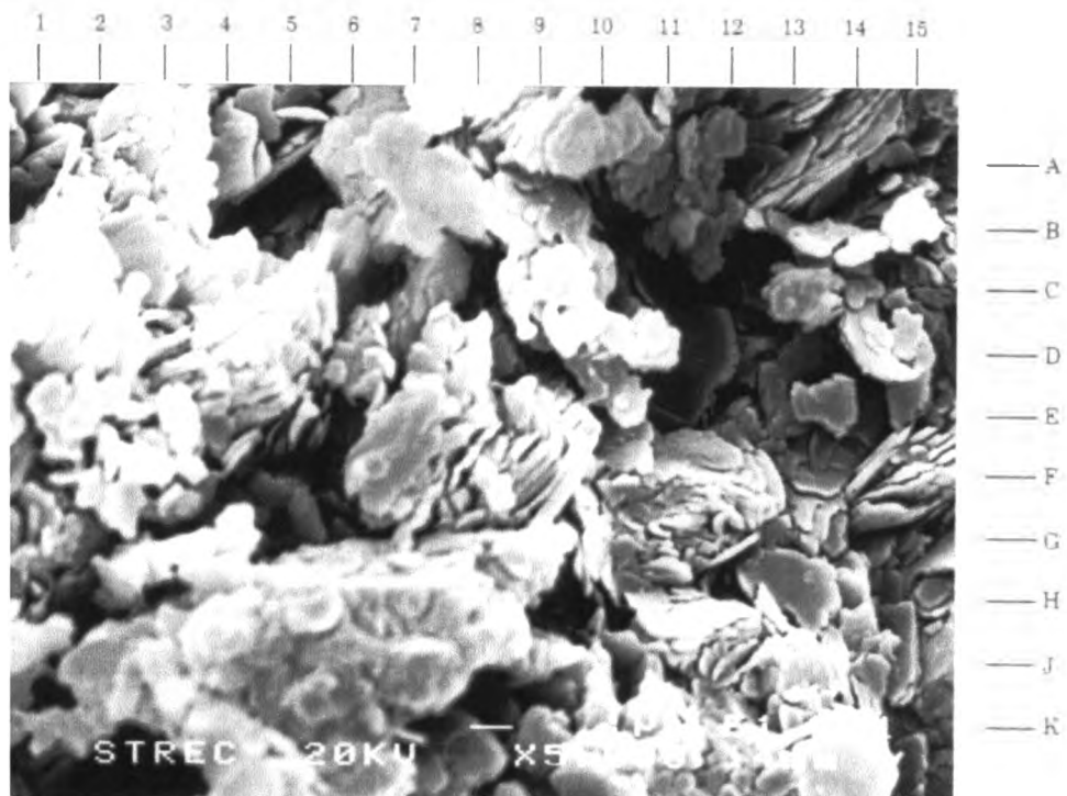
Fig. 3.30 Scanning electron micrograph of weathered rhyolitic tuff showing the mixtures of kaolinite (A7, J6) and illite (F7, F9) (see EDS curves in Figures 3.34 and 3.35).
