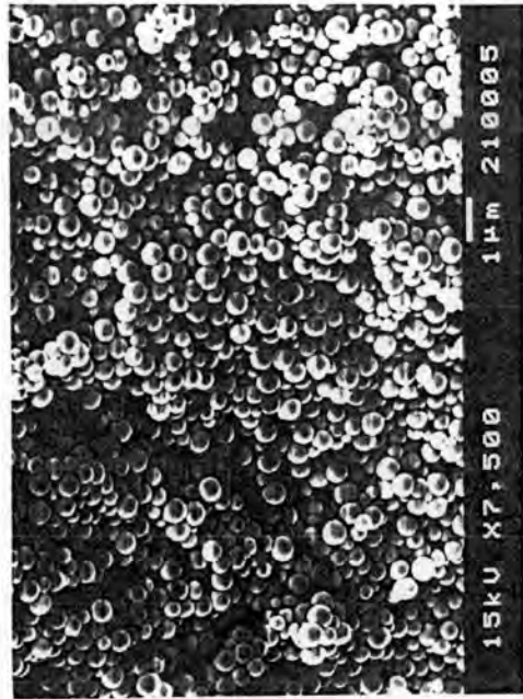
Figure 4.34 SEM micrographs for PSD measurement of poly(styrene-co-methyl methacrylate) synthesized in 70/30 EtOH/H 2 O controlled by 8 wt% PVP K-30
