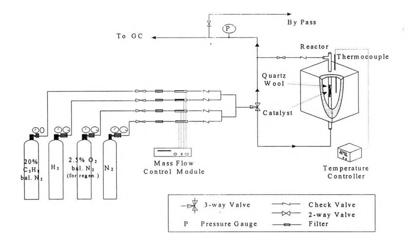
Figure 3.1 Schematic diagram of experimental equipment.
