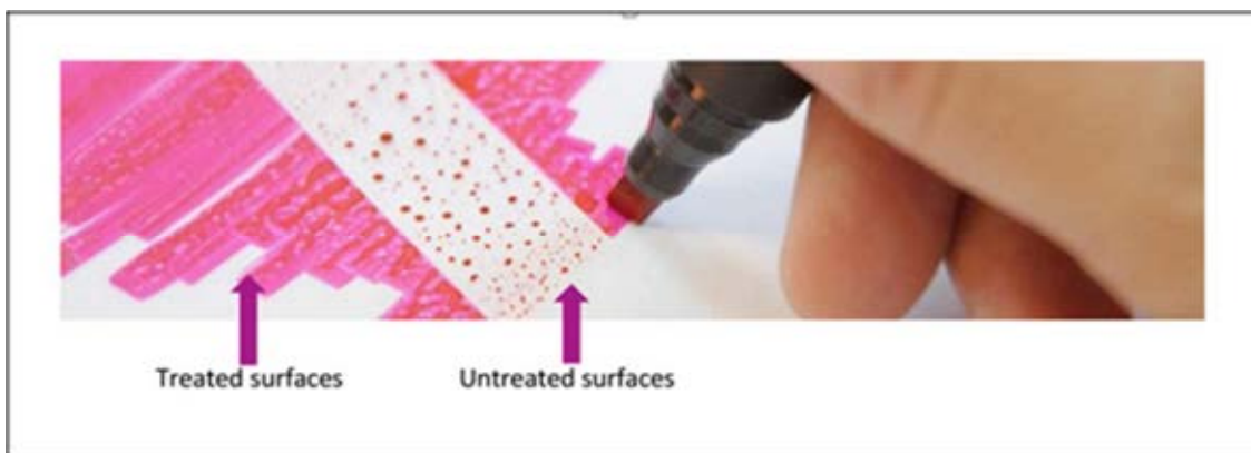
Figure 21. Comparison between treated and untreated corona treatment on PET film by corona-check dyne test pen at 50 dyne/cm
