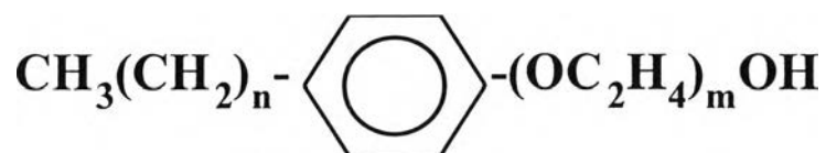
Figure 2.1 Molecular structure of polyoxyethyl phenylether, where n is the number of alkyl groups and m is the number of alkoxy groups
