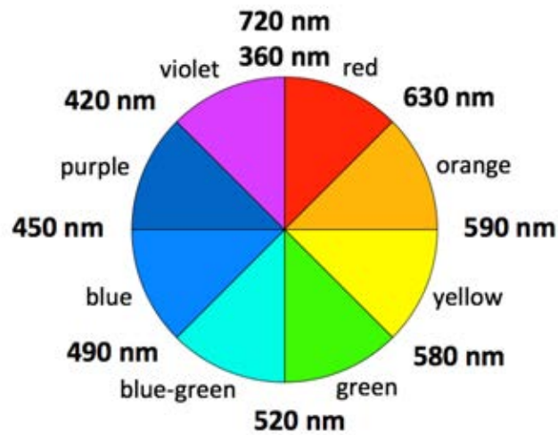
Figure 13 : Color wheel with wavelengths from the work of Tem5psu (Tem5psu, 2017).
