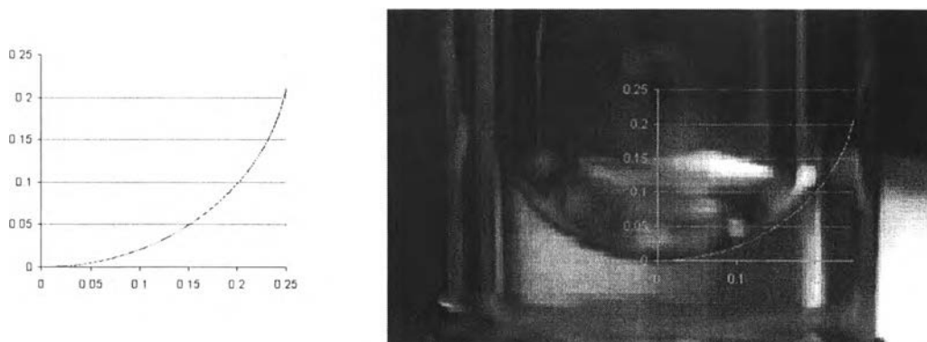
Figure E.1 Comparison of meniscus resulted from the model and experiment for vertical annular tube at inner/outer tube of 7/10 mm.
