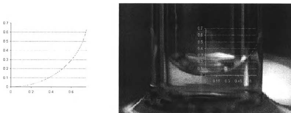
Figure E.2 Comparison of meniscus resulted from the model and experiment for vertical annular tube at inner/outer tube of 10/15 and 15/20 mm.
