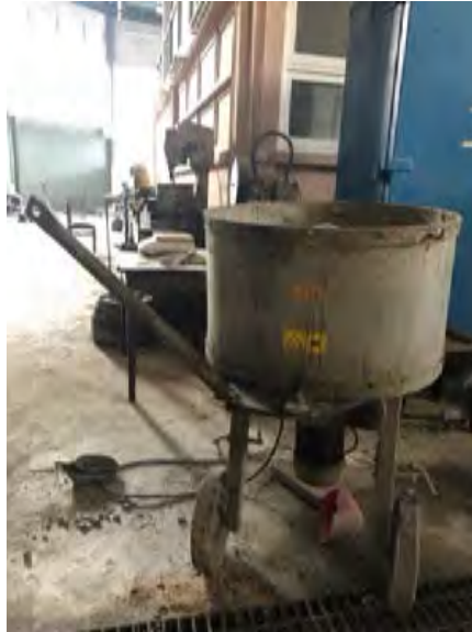
Figure 3.2 Concrete mixer machine
