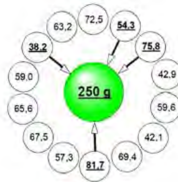
Figure 8: Logic of weight controlled filler (Fellows, 2017)
