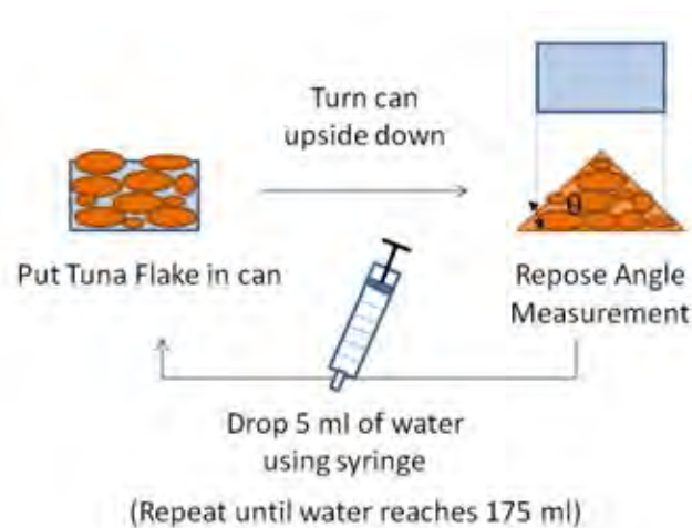
Figure 39: Repose angle measurement
