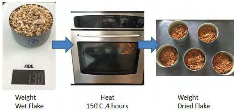
Figure 29: Moisture measurement procedure
