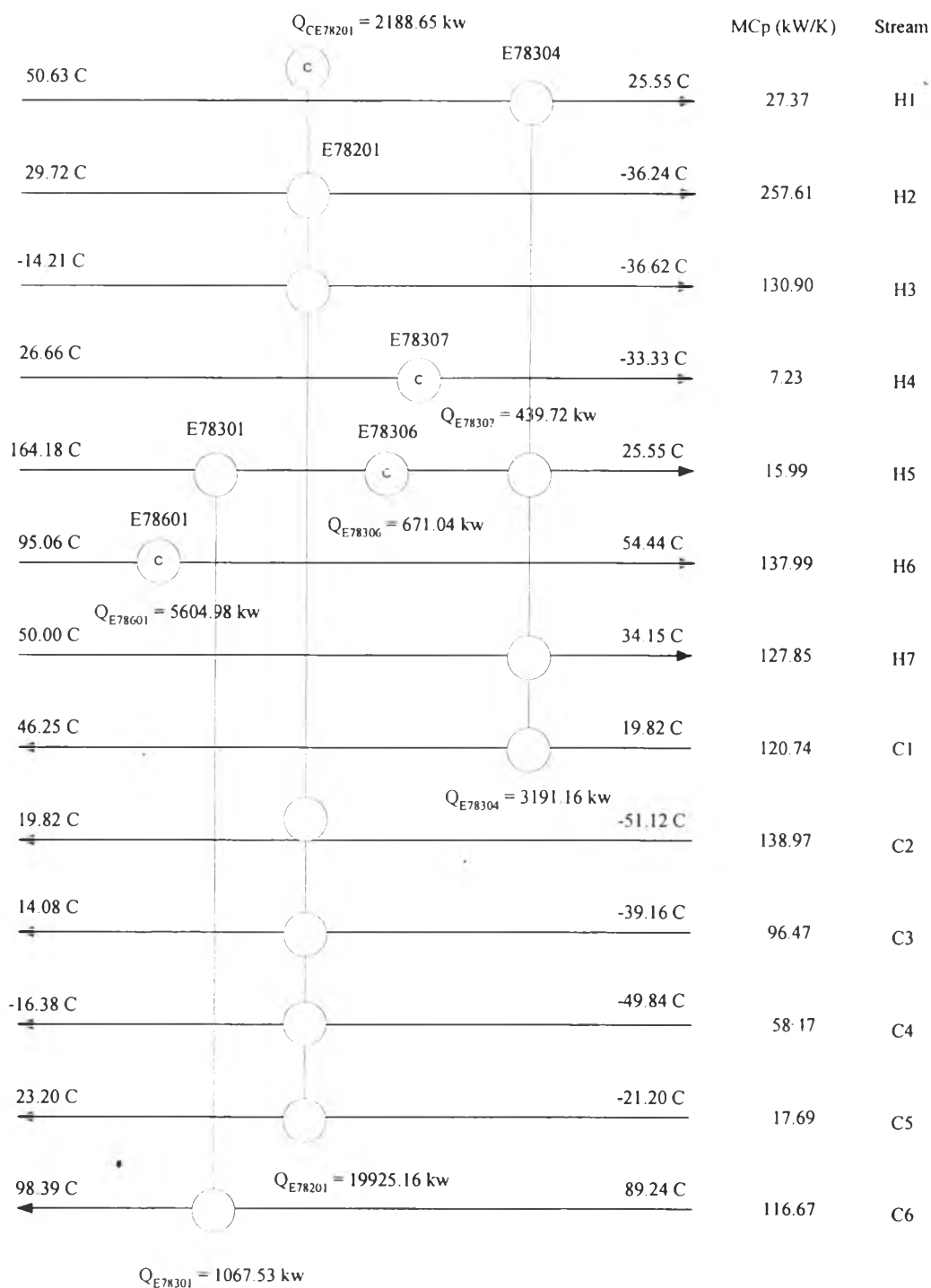
Figure 4.5 Grid diagram of existing gas separation unit (design case).
