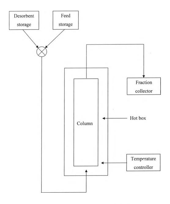
Figure 3.1 Experimental set-up of the pulse test unit.
