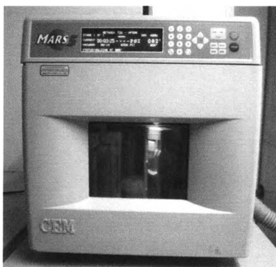
Figure 3.1 A CEM (Matthews, NC, USA) MAR-5 HP-500 microwave system.
