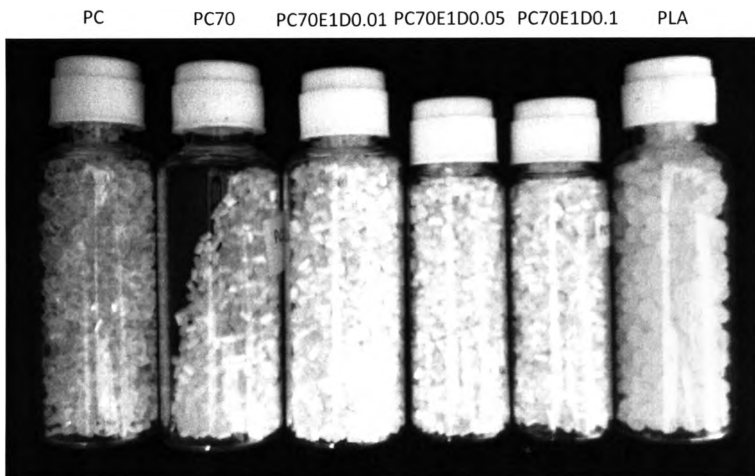
Figure 7.2 Pellets of PC, PLA and PC/PLA/EAA/DBTO blends.
