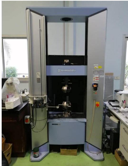
Figure 5 Universal testing machine (SHIMADZU AGS-X 100kN model, Japan)
