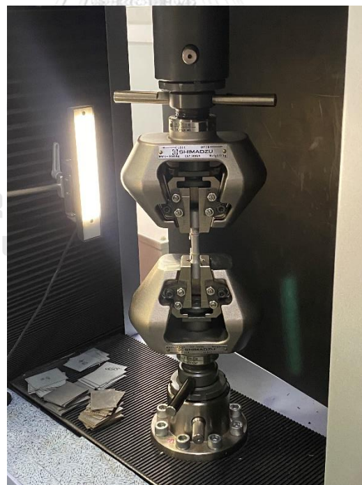
Figure 6 The grip of universal testing machine held the sample.
