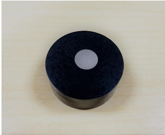
Figure 8 Prepared sample after polishing in bakelite moulding
