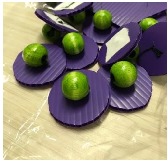
Figure 8 18-mm diameter spherical markers with adhesive tape
