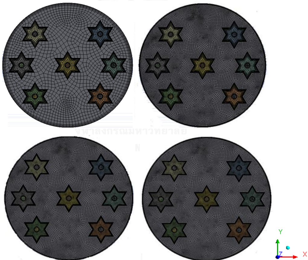
Figure 3.8 The meshed geometry of the star-shaped microfiltration membrane.
