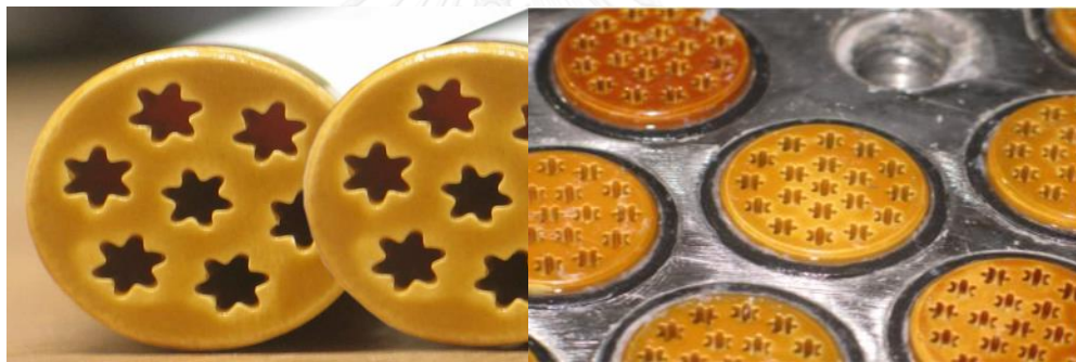
Figure 2.4 Geometry of star shaped microfiltration membrane [4]
