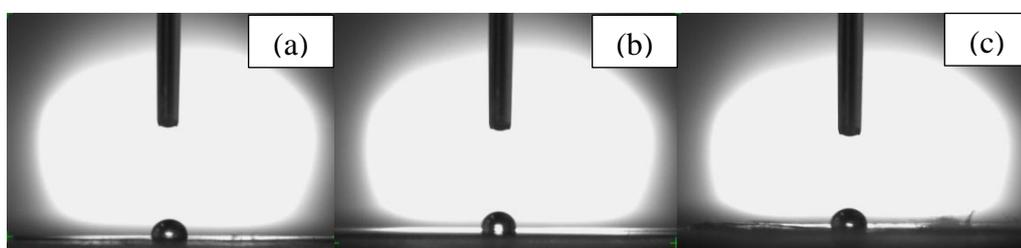
**Figure 5.12** Photograph of water contact angle on s-BPDA/NTDA(70/30)-ODA copolyimide surface at various content of silane coupling agent in copolymer : (a) PI, (b) PI with 0.5 %wt of silane and (c) PI with 1.0 %wt of silane.
