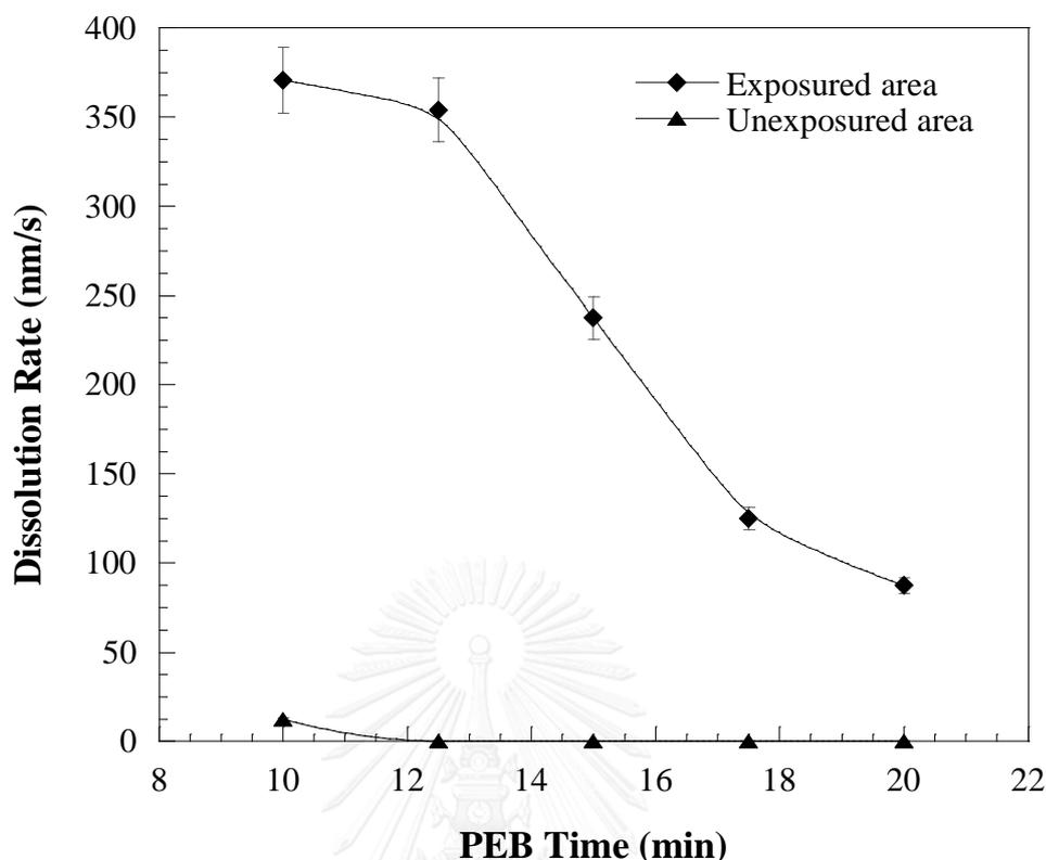
**Figure 5.9** Relationship between the PEB time and dissolution rate of a copolyimide containing 20 wt% nifedipine at 140°C PEB temperature.
