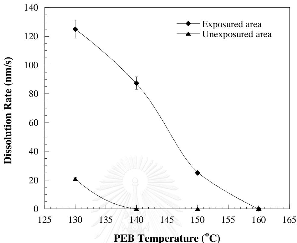
**Figure 5.8** Relationship between the PEB temperature (for 20 min) and dissolution rate of a copolyimide containing 20 wt% nifedipine.
