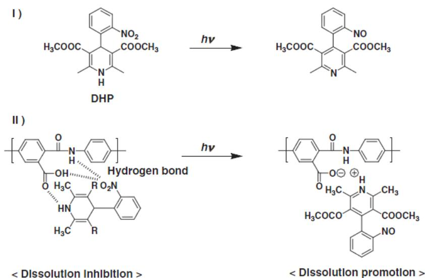
**Figure 2.11** Dissolution inhibition mechanism with DHP [17].
