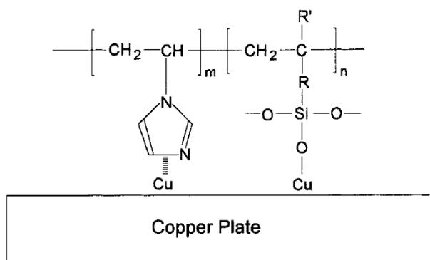
**Figure 5.13** The interaction of the interaction between silane-modified PI and copper.
