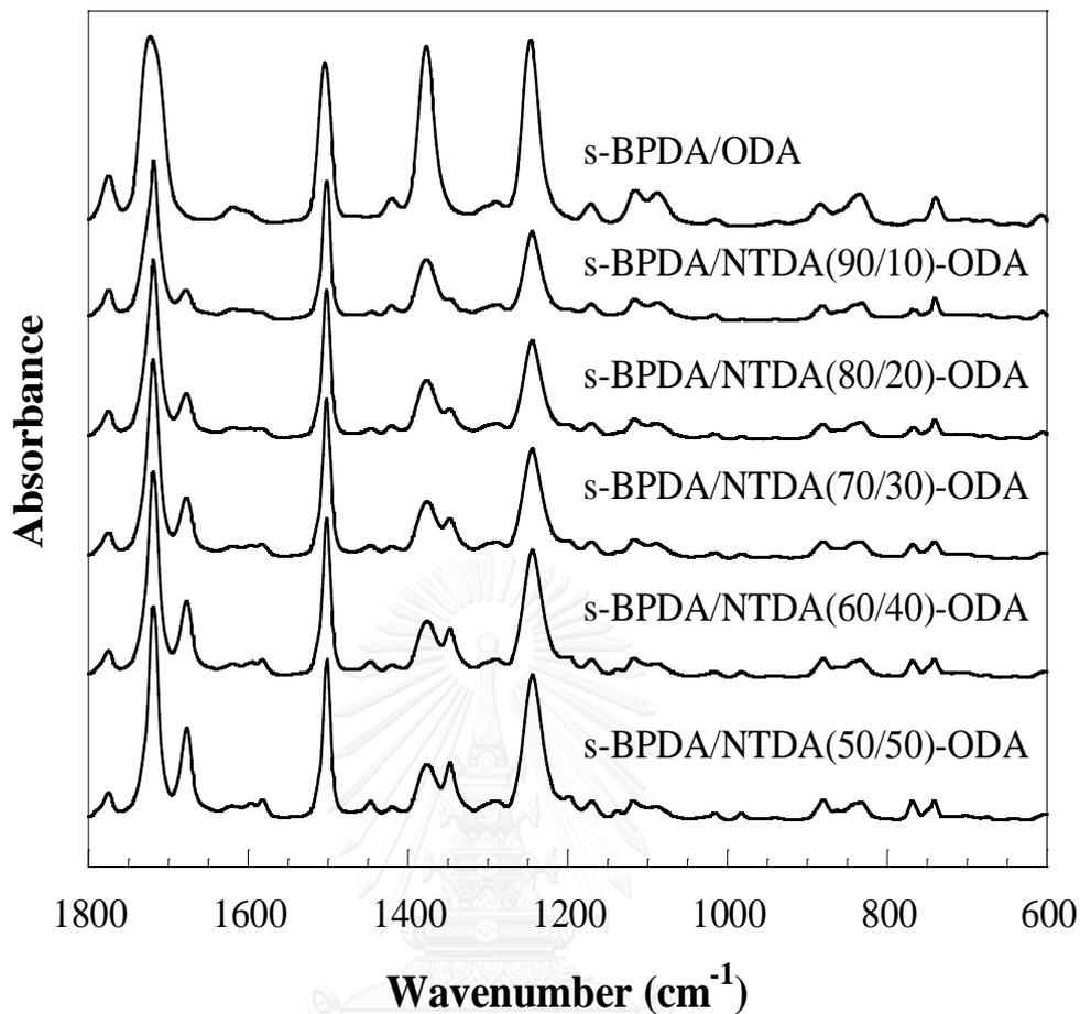
**Figure 5.2** FTIR spectra of s-BPDA/ODA polyimide and its copolyimides with NTDA.
