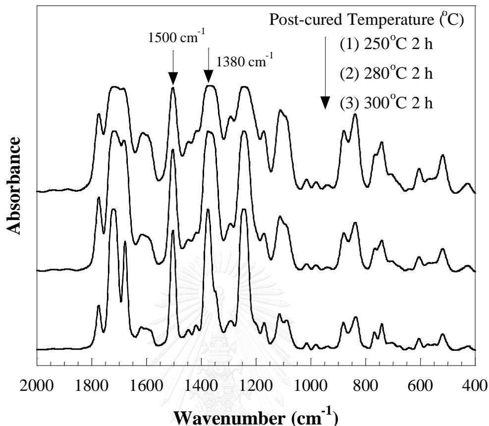
**Figure 5.1** IR spectra of the s-BPDA/NTDA(70/30)-ODA copolyimides at curing 100°C 1 h followed post-cured at temperature: (1) 250°C for 2 h, (2) 280°C for 2 h, (3) 300°C for 2 h.
