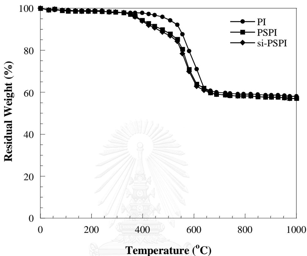
**Figure 5.19** TGA thermograms of copolyimide film (PI) photosensitive copolyimide film (PSPI) and silane-containing photosensitive copolyimide film (si-PSPI).
