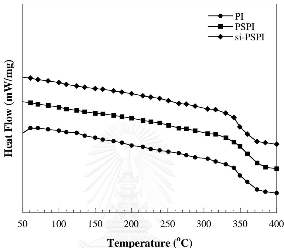
**Figure 5.18** DSC thermograms of copolyimide film (PI) photosensitive copolyimide film (PSPI) and silane-containing photosensitive copolyimide film (si-PSPI).
