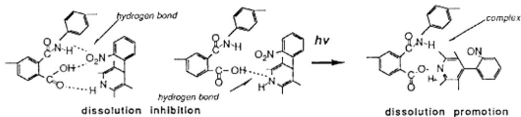
**Figure 3.5** Nifedipine photoconverted quantitatively to NDMPy in a polyimide precursor film [20].
