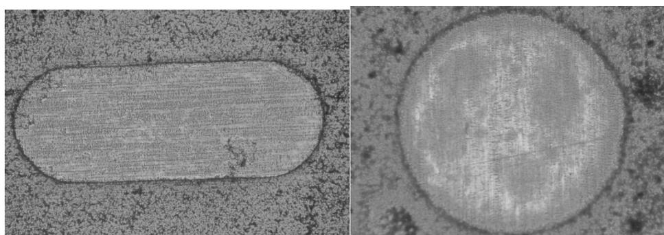
**Figure 5.17** Optical micrographs of positive-type fine patterns obtained from our silane-containing PSPI (30  $\mu\text{m}$  thick, nifedipine 20 wt%).
