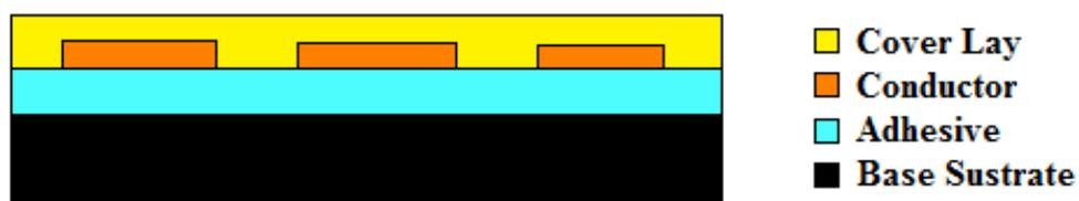
**Figure 2.3** Flexible-circuit make up [21].
