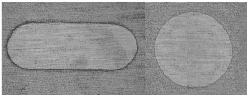
**Figure 5.11** Optical micrographs of positive-type fine patterns obtained from our PSPI (30  $\mu\text{m}$  thick, nifedipine 20 wt%).
