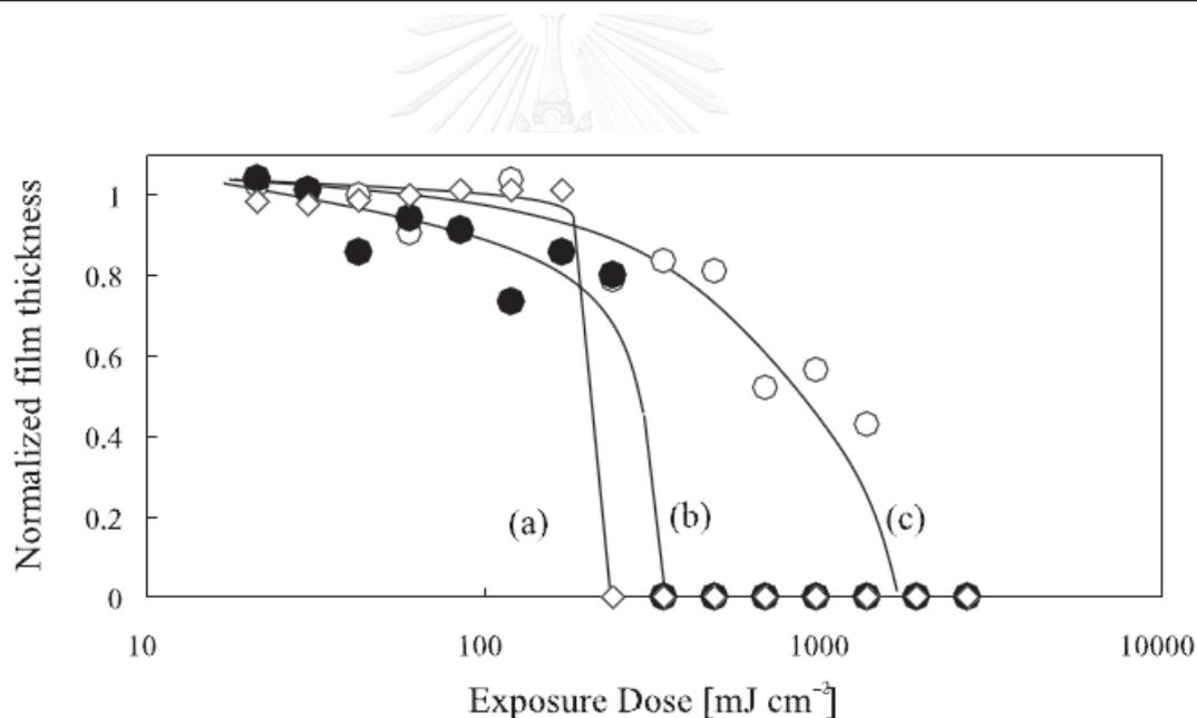
**Figure 3.1** Photosensitivity curves for PSPI-5 film as a function of DNQ content: (a) 9.09 wt% (10 phr), (b) 16.6 wt% (20 phr), and (c) 23.1 wt% (30 phr) [1].
