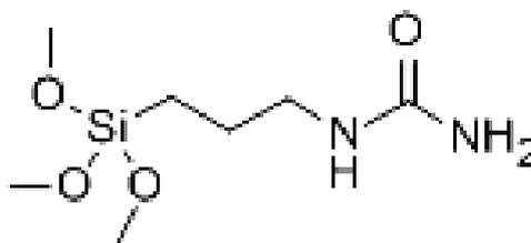
**Figure 2.16** Chemical structure of 1-[3-(Trimethoxysilyl)propyl]urea [48].
