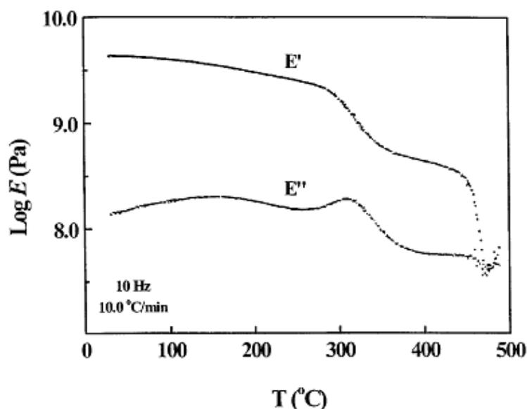
**Figure 3.3** Variations of dynamic moduli (storage modulus  $E'$  and loss modulus  $E''$ ) of BPDA-ODA polyimide film as a function of temperature. The employed frequency and heating rate were 10 Hz and 10.0 K/min, respectively [6].
