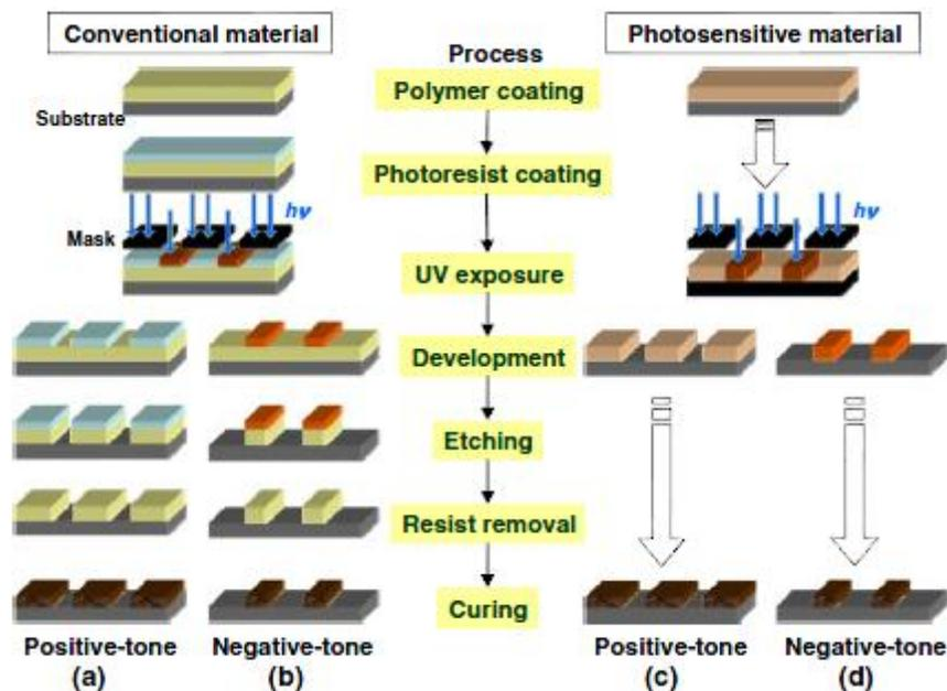
**Figure 2.9** Photolithographic patterning processes in conventional methods using photoresists (a & b) and in advanced methods using photosensitive materials (c & d) [17].
