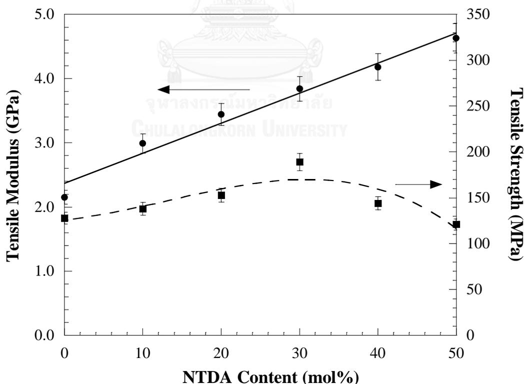
**Figure 5.5** Tensile properties of the s-BPDA/ODA polyimide and its copolyimides.
