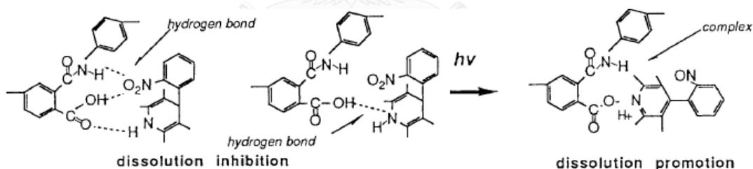
**Figure 5.6** Chemical reactions or interactions occur through the exposure process between a polyimide precursor and nifedipine.
