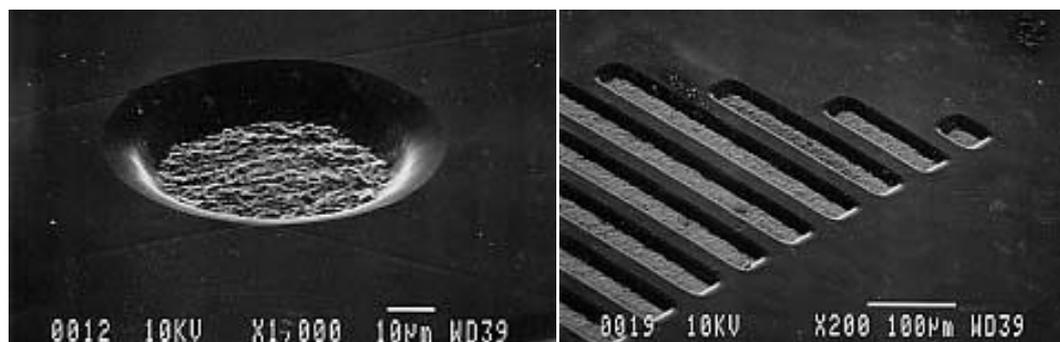
**Figure 3.2** SEM photographs of positive-tone fine patterns obtained from PSPI-5 (10  $\mu\text{m}$  thick, DNQ: 9.09 wt%): (a) dot and (b) line and space patterns. Developed using a 3 wt% NaOH aqueous solution at 40°C for 150 s and rinsed in water at 40°C for 120 s after irradiation of 1500  $\text{mJ}/\text{cm}^2$  [1].
