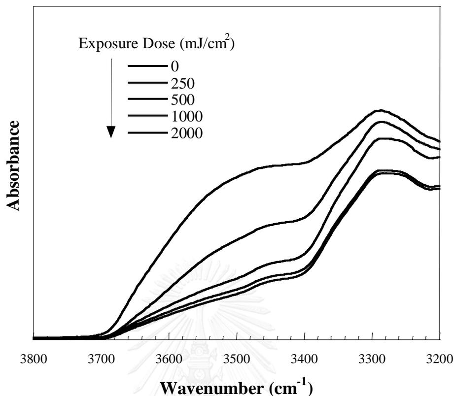
**Figure 5.7** Change in IR spectra of PSPI film with an increase in UV exposure doses.
