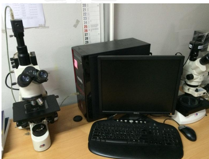
Optical microscope, Seek Inter Co., Ltd., model SK-XJM series with video recorder
