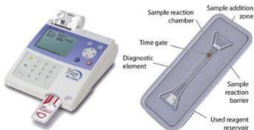
Figure 1.9 Example of commercially available LOC representing the various parts of tasks on the limited space device[10]
