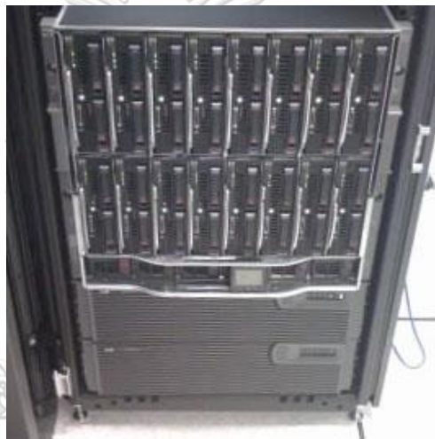
Fig. 2: HP BladeSystem c7000 enclosure (populated with 16 blades), with two 3U UPS units below [20].
