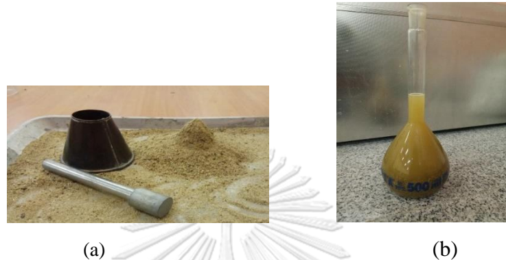
Figure 22: Performance test (a) saturated surface dry of fine aggregate and (b) specific gravity of fine aggregate
