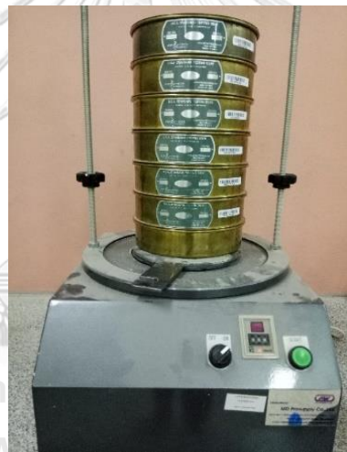
Figure 21: Mechanical sieve shaker
