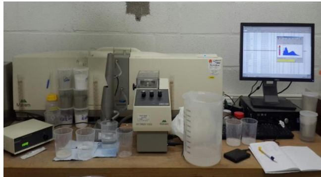
Figure 18: Laser particle size analyzer machine
