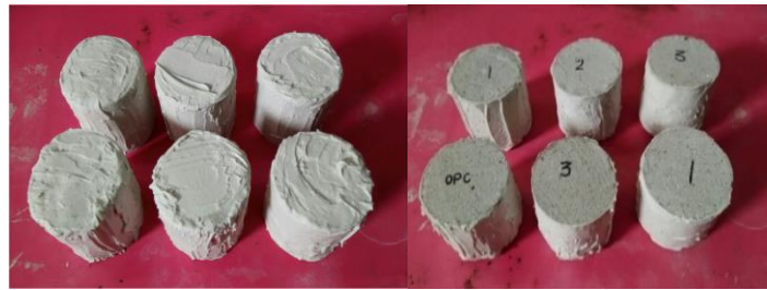
Figure 29: Preparing specimens for accelerated carbonation
