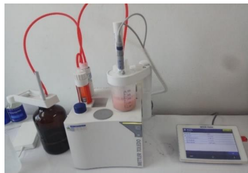
Figure 28: Measuring the total \text{Cl}^- content
