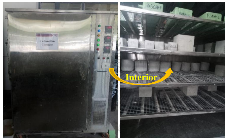
Figure 30: Specimens placed in carbonation chamber
