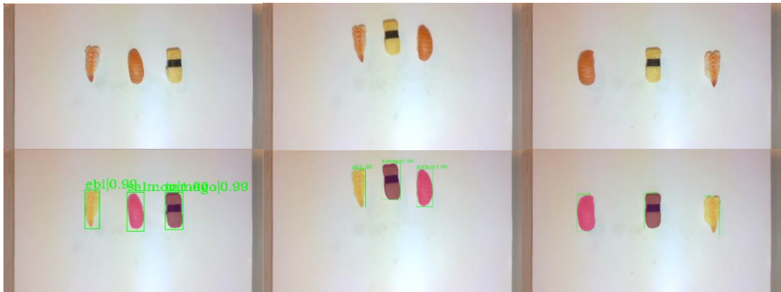
Fig. 48 Examples of the sushi set detections in different image resolutions: 320x180 (Left), 848x480 (Middle), and 1920x1080 (Right)
