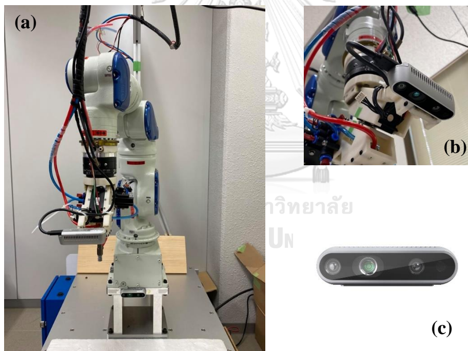
Fig. 20 Manipulator and the camera used for computer vision: (a) Motoman SIA5F Manipulator, (b) Depth camera mounted at the end-effector, (c) Intel RealSense D435i Depth camera
