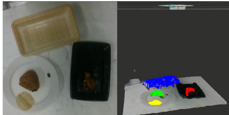
Fig. 52 RGB frame of the depth camera (Left) and extracted point cloud visualization (Right)
