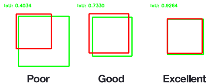
Fig. 3 IoU examples. Here the red bounding box represents ground-truth while the green bounding box represents prediction by the model.
