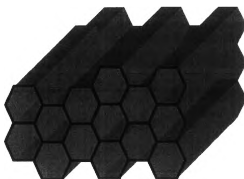
Figure 2.12 Hexagonal mesoporous structure.
