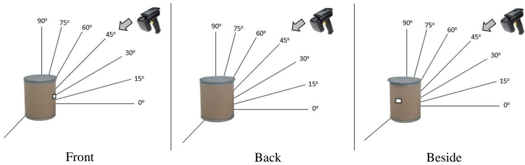
Figure 28 Reading position of SM tank with metal case
