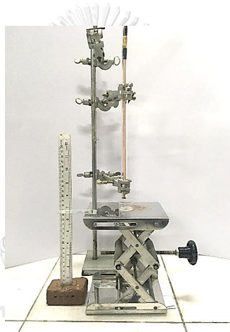
Figure 36 The experiment setup for investigating the probe voltage reflection coefficient spectrum responses.
