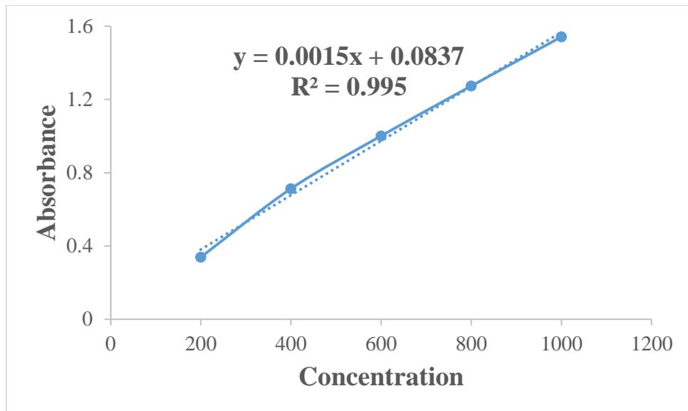
**Figure 4.14** Calibration curve of erythromycin standard solutions
