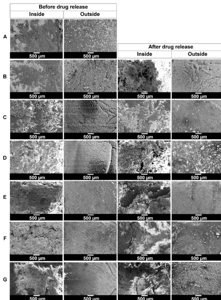
SEM images of poly(methyl methacrylate) spacer impregnated with (A) none, (B) vancomycin (VAN-PMMA), (C) vancomycin-loaded rice granules (VAN-RG-PMMA), (D) vancomycin-loaded calcium citrate particles (VAN-RG-PMMA), (E) erythromycin (ERY-PMMA), (F) erythromycin-loaded ethyl cellulose particles (ERY-EC-PMMA), and (G) erythromycin-loaded poly(lactic-co-glycolic acid) particles (ERY-PLGA-PMMA). The green arrows indicate the poly(methyl methacrylate) particles.
