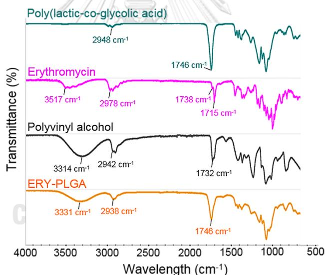
**Figure 4.16** FTIR spectra of poly(lactic-co-glycolic acid) polymers (green line), erythromycin (pink line), polyvinyl alcohol (grey line), and erythromycin-loaded poly(lactic-co-glycolic acid) particles (orange line)
