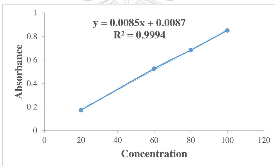
**Figure 4.10** Calibration curve of erythromycin standard solutions
