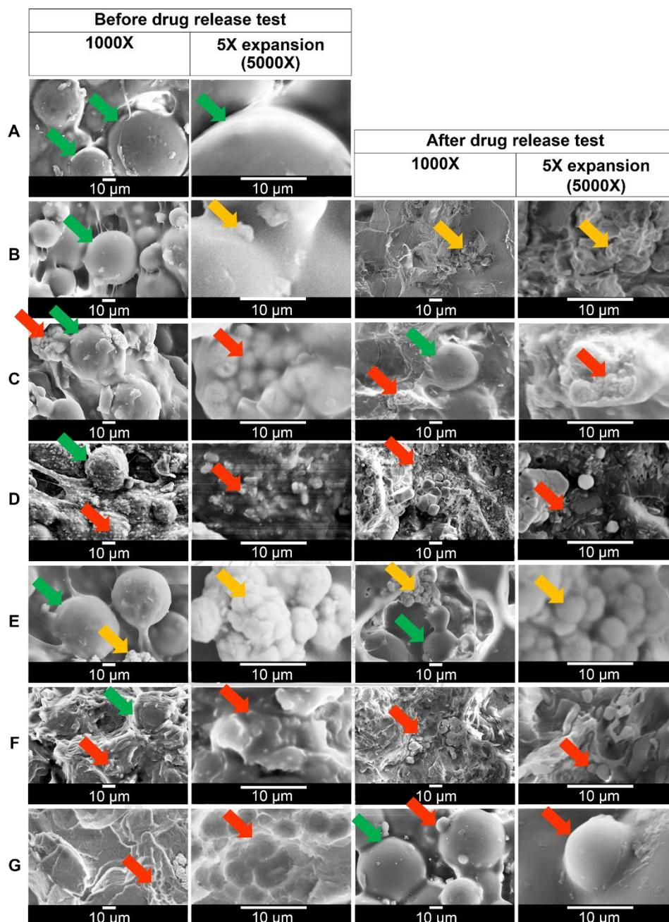
**Figure 4.19** SEM images of poly(methyl methacrylate) spacer impregnated with (A) none, (B) vancomycin (VAN-PMMA), (C) vancomycin-loaded rice granules (VAN-RG-PMMA), (D) vancomycin-loaded calcium citrate particles (VAN-RG-PMMA), (E) erythromycin (ERY-PMMA), (F) erythromycin-loaded ethyl cellulose particles (ERY-EC-PMMA), and (G) erythromycin-loaded poly(lactic-co-glycolic acid)
