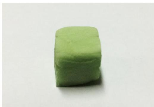
**Figure 4.18** PMMA composite in a cubic shape of 1x1x1 cm<sup>3</sup>
