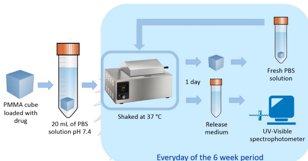
**Figure 3.2** Drug release test
