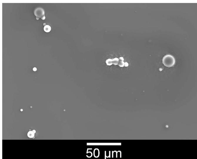
**Figure 4.15** SEM images of erythromycin-loaded poly(lactic-co-glycolic acid) particles
