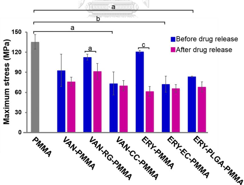
**Figure 4.22** Compressive strengths of all PMMA composites measured in maximum stress (MPa) before and after drug release test for 42 days. Significant differences between the tested groups are labeled with a, b, and c for level of certainty of 0.05, 0.01, and 0.001, respectively.
