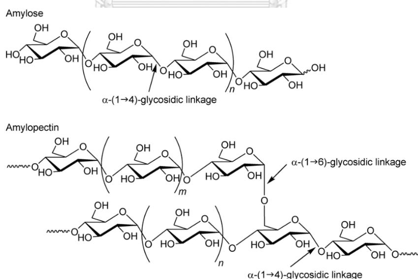
**Figure 2.5** Structure of amylose and amylopectin
