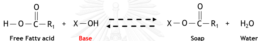
Figure 2 Saponification reaction of free fatty acid with alkali catalyst
