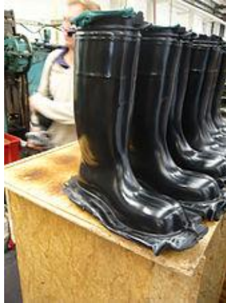
Figure 2.6 Compression molded (cured) rubber boots [22].
