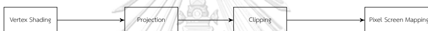
Figure 2.6: Geometric processing contains four sub-stages; vertex shading, projection, clipping and screen mapping.
