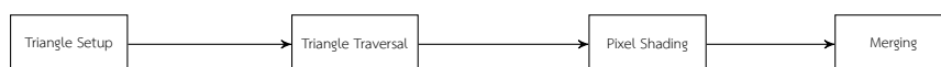
Figure 2.7: Rasterization substage contains triangle setup and triangle traversal. Pixel processing substage contains pixel shading and merging.
