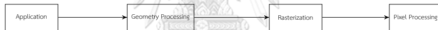
Figure 2.4: The graphics rendering pipeline contains four stages; application, geometry processing, rasterization, pixel processing.
