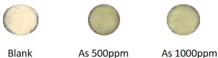
Figure 3.1 The visual image of the detection zone for the determination of As(III) at the concentration of 0, 500 and 1,000 ppm using 1,000 ppm Ag(I) as a color reagent with a reaction time of 10 min.
