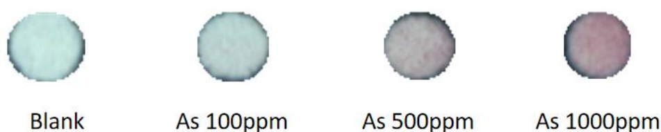
Figure 3.2 The visual image of the detection zone for the determination of As(III) at the concentration of 0, 100, 500 and 1,000 ppm using 1,000 ppm Au(III) as a color reagent with a reaction time of 10 min.
