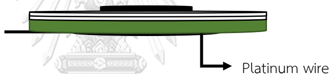
Fig. 30 platinum wire attachment for an electrical connection
