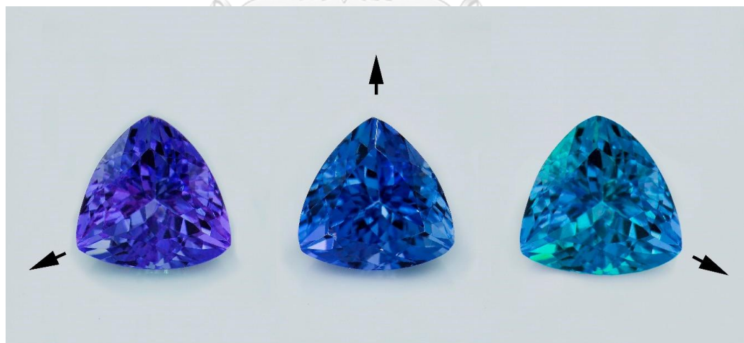
Figure 1 Trichroism of a natural tanzanite rotated in three directions showing violet, blue, and green pleochroic colors (Photo by T. Sripoonjan, GIT).
