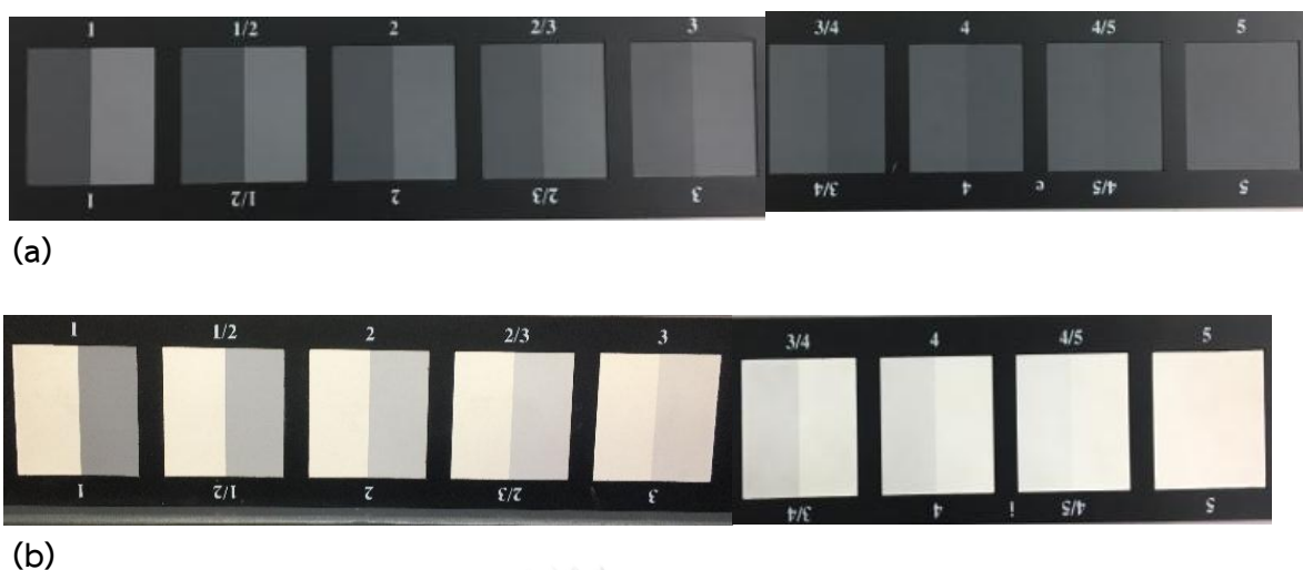
Figure 3.3 (a) Gray scale for Assessment color change (ISO 105-A02-1993) and (b) Gray scale for Assessment staining (ISO 105-A03-1993)
