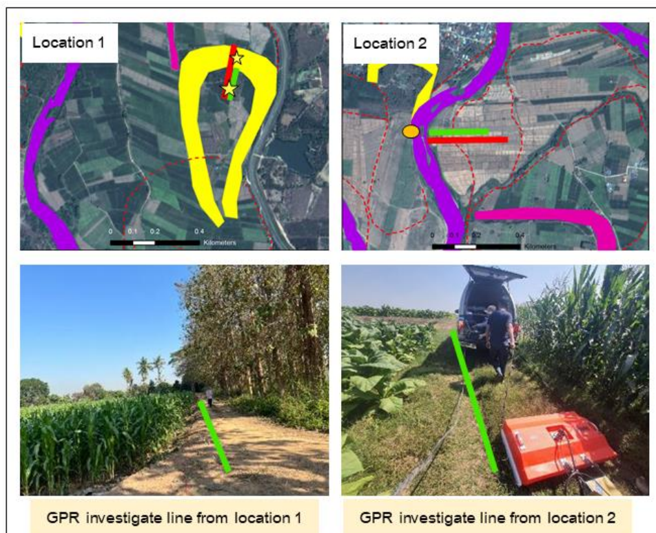
Figure 32 The GPR investigation lines from 2 locations in fieldwork investigation.
