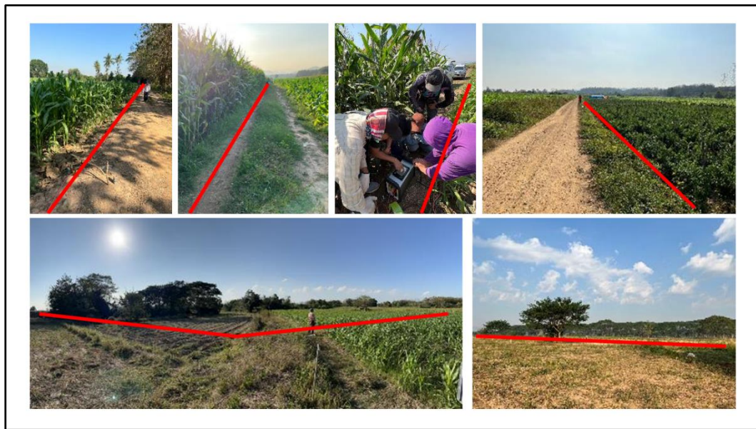
Figure 33 Resistivity investigation lines (Red lines) in six locations where located of paleochannels, floodplains and point bars on the map on figure 30. Location 1(A), Location 2 (B), Location 3 (C), Location 4 (D), Location 5 (E) and Location 6 (F).
