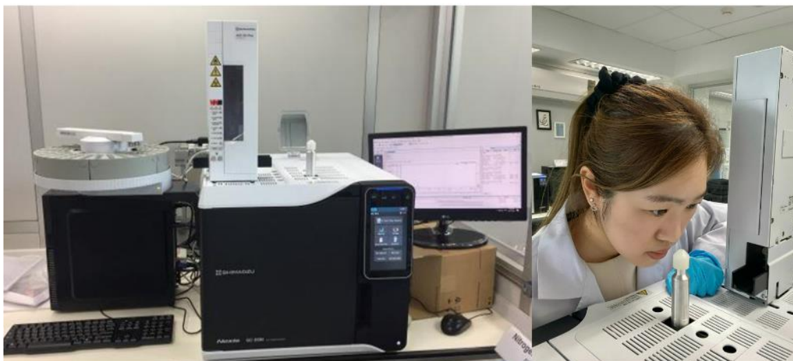
Figure 3.4 Determination of aroma compounds using gas chromatography-olfactometry/ flame-ionization detection (GC-O/FID)
