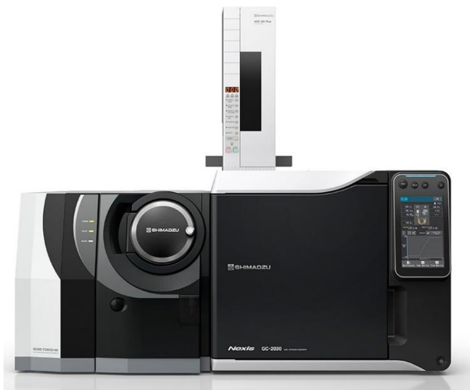
Figure 3.5 Determination of volatile compounds using gas chromatography-mass spectrometry (GC-MS)
