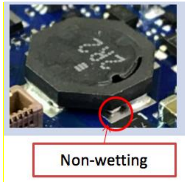
Figure 10: The sample of Non-wetting defect on L7 location (2)
