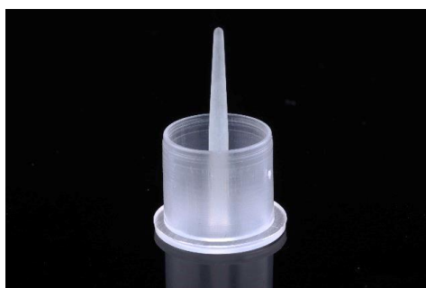
Figure 17 demonstrates the plastic cap with a hole in the bottom which a glass fiber post was placed.
