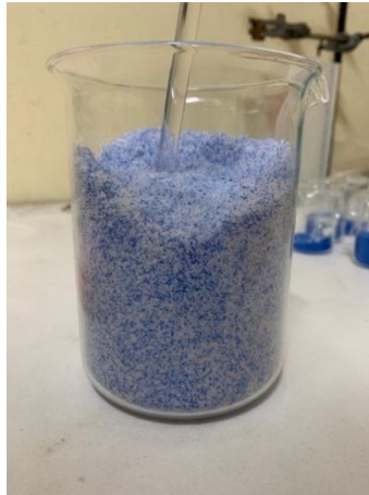
Figure 3.6 A mixture of 5% of 0.25-0.5 mm MP in 0.5-1.0 mm sand
