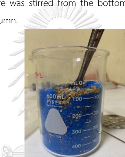
Figure 4.27 The mixture of 15% MP 0.5-1.0 mm in sand 2.0-4.0 mm
