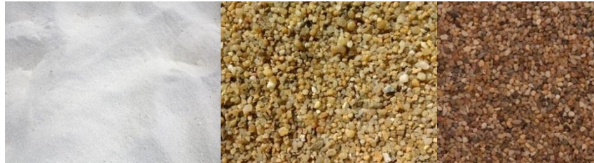
Figure 3.3 The sands (0.5-1.0, 1.0-2.0 and 2.0-4.0 mm respectively)
