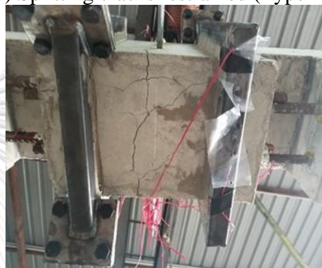
(c) Splitting cracks initiated and propagated along lap splice (Type-II)
