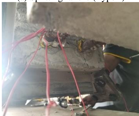
(c) Splitting cracks initiated and propagated along lap splice (Type-II)
