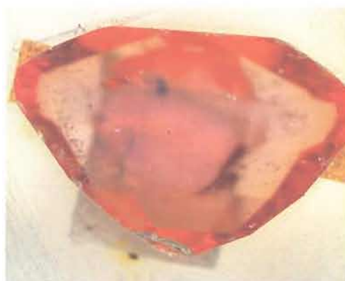
Figure 4.22: An orange Songea sapphire (SGDH09) reportedly underwent a Be-treatment was cut in half and a five-point profile was analyzed across the cut surface using LA-ICP-MS. (Photo by Lomthong, KU)
