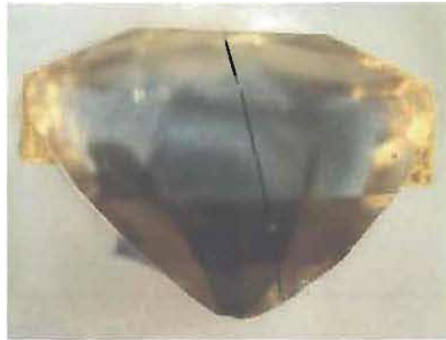
Figure 3.5: A natural blue sapphire (PPBS1) reportedly heat-treated with Be under unknown condition by a Thai heater and cut in half. The sample shows a thi surface-related yellow rim surrounding the blue core. High magnification reveals that the blue core contains oriented blue dots probably resulting from partial dissolution of rutile needles. A five-point profile was analyzed across the cut surface with two points in the surface-related yellow zone (rims) and three points in the blue core. (Photo by Lomthong, KU)
