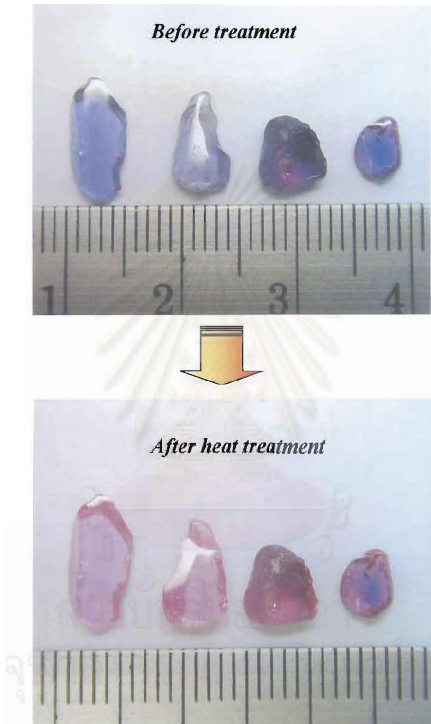
Figure 8.1a: Heat treatment of Madagascan sapphires to improve their color and clarity. (Photos by Somboon, GIT)
