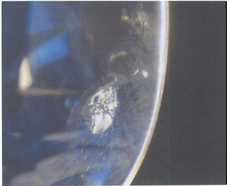
Figure 7.53: Shiny thin-film tension disc is obvious indication of heating.
