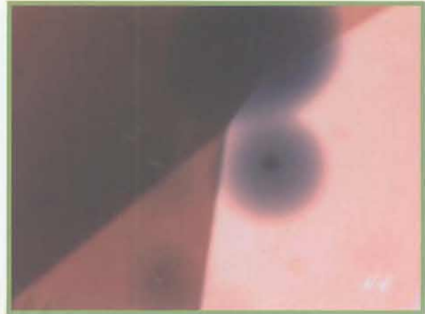
Figure 5: Internal diffusion of Ti from rutile inclusions into the corundum lattice showing the blue haloes. (Photo by Häger)
