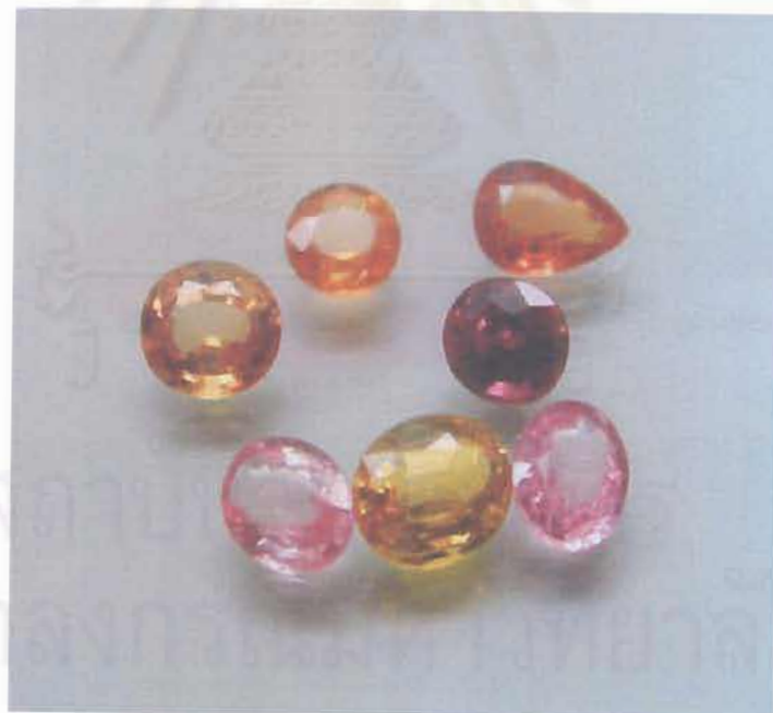
Figure 8.23: Multitude of colours in Be diffusion-treated sapphires such as pink-orange, orange, yellow and orangey red. (Photos by Somboon, GIT)
