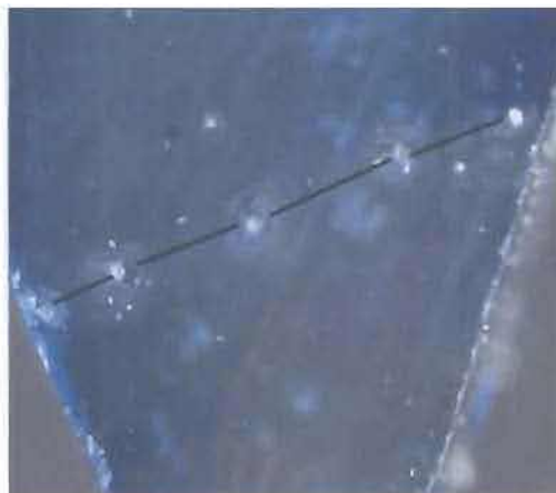
Figure 3.1: A natural blue sapphire (DIF1) reportedly underwent a ‘classical’ heat-treatment was cut in half. A five-point-profile was analyzed across the cut surface using LA-ICP-MS. (Photo by Lomthong, KU)
