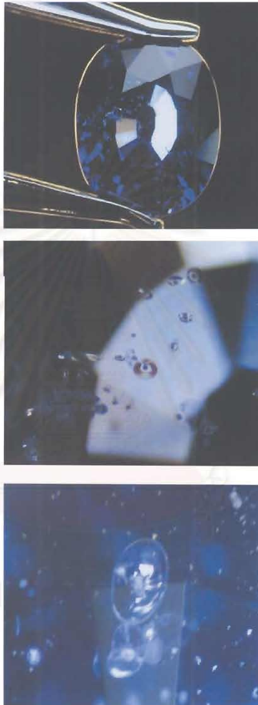
Figure 8.9: A 4.69 ct Mada sapphire showing rather clear stone. The stone shows obvious thin-film tension disc due to heating. (Photos by Somboon, GIT)
