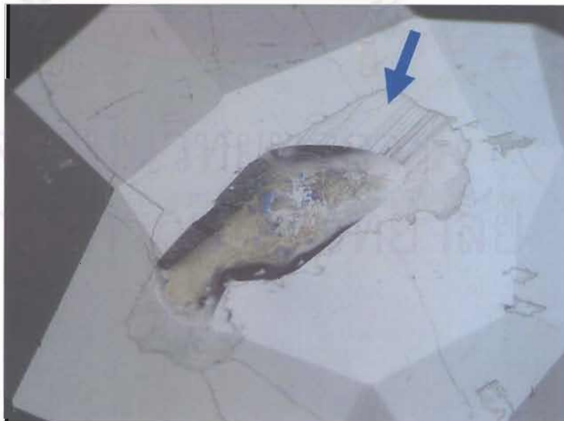
Figure 8.39: The cavity-filled Pb-glass (arrow) displays high luster but is poorly polished on the surface. (Photos by Leelawathanasuk,GIT)
