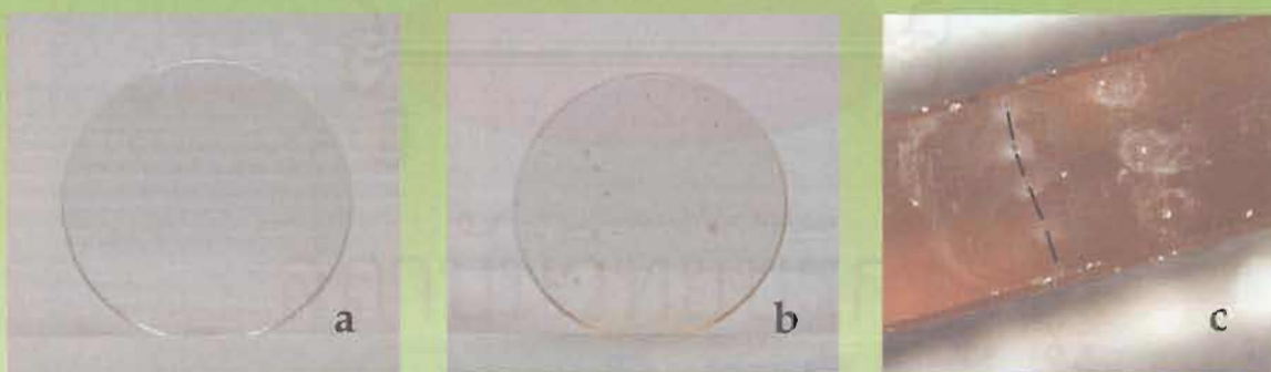
Figure 16: Photos of the 13.51 ct disc of colourless 'watch glass' sapphire (WG01) before treatment (a), and pale brown throughout the entire disc after Be-treatment under unknown conditions (b). After the treatment, a five-point-profile (c) was analysed across the 1.25 mm thick cut surface using LA-ICP-MS
