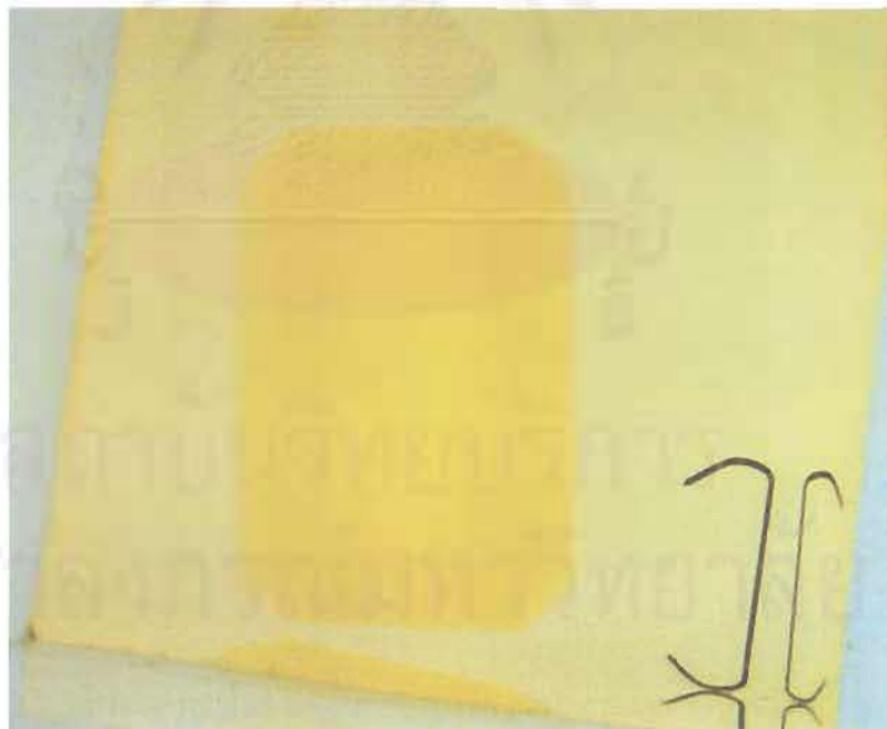
Figure 8.25: Surface-related colour zone is a diagnostic features of yellow Be-diffusion treated sapphires. (Immersion: Photos by Leelawatanasuk, GIT).
