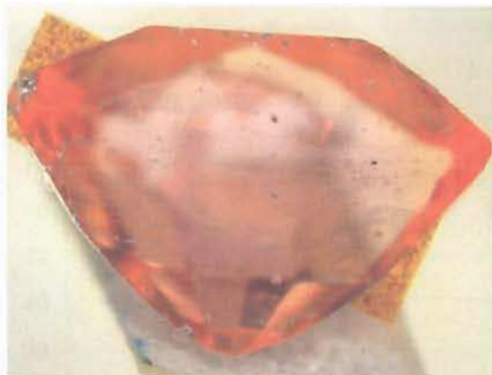
Figure 4.26: An orangey pink Madagascan sapphire (WSMDIF7) reportedly underwent a Be-treatment was cut in half and a five-point profile was analyzed across the cut surface using LA-ICP-MS. (Photo by Lomthong, KU)
