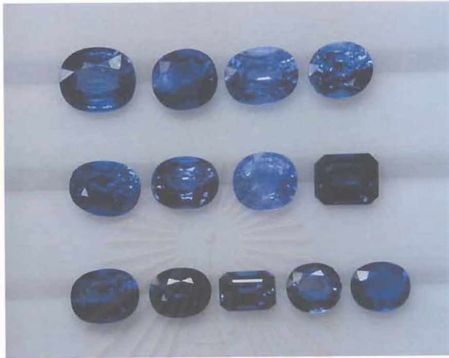
Figure 7.1: Series of un-heated Ilakaka blue sapphires (13 samples) varying from pale to very dark blue (with the courtesy of World Sapphires Co. Ltd.)
