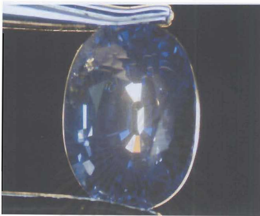
Figure 7.51: This 2.74 ct Myanmar blue sapphires showing strong tension disc due to heating.
