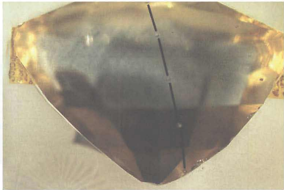
Figure 25: Photo of a blue sapphire (PPBS1) reportedly heat treated with Be under unknown conditions by a Thai heater. The sample shows a thin surface-related yellow rim surrounding the blue core. High magnification reveals that the blue core contains oriented blue dots probably resulting from partial dissolution of rutile needles. A five-point profile was analysed across the cut surface with two points in the surface-related yellow zone (rims) and three points in the blue core. (Photo by Somboon, GIT and Lomthong, KU)
