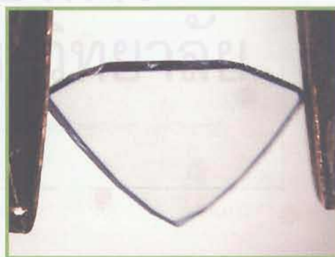
Figure 4: Slice of colourless sapphire with blue rim caused by external diffusion of Ti into the stone; 4 × 7 mm. (Immersion, photo by Häger)
