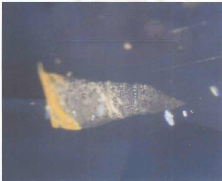
Figure 7.12: Yellowish orange colour impurity in healed fractures is also suggesting un-heated feature
