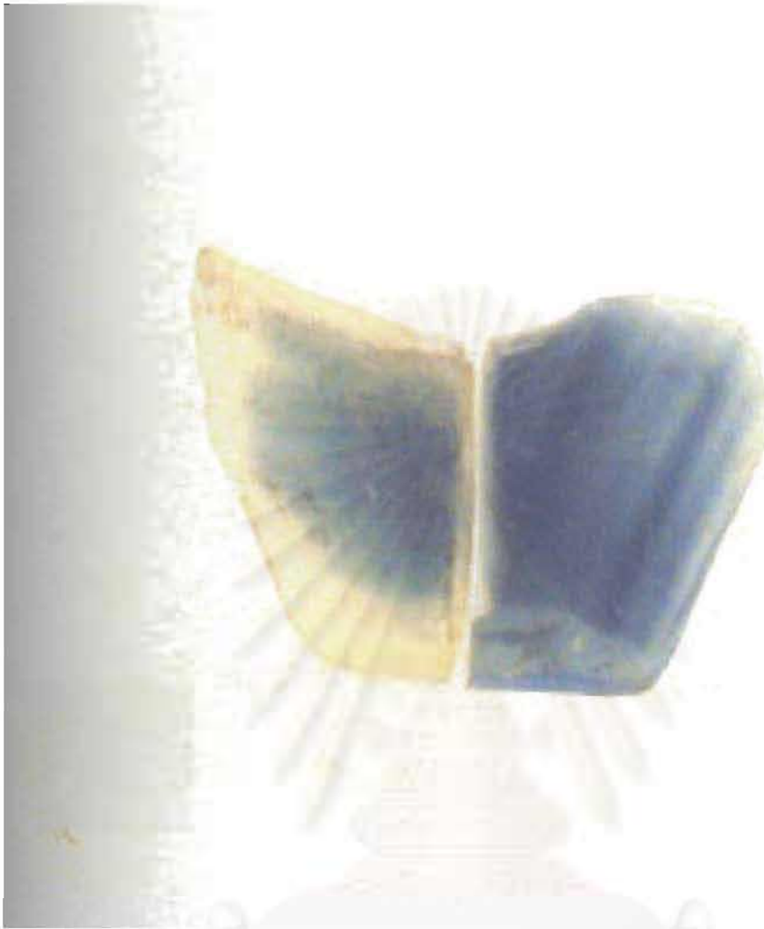
Figure 3.11: A natural blue sapphire was cut in half; the left half was heat-treated with ground chrysoberyl in a crucible while the right half was heated in another crucibles without chrysoberyl. The heating condition for both crucibles was 1,750^{\circ}\text{C} for 30 hours in air. After heat treatment the left half shows obviously surface-related yellow rim whereas the right half is blue throughout the stone. (Photo by Häger)
