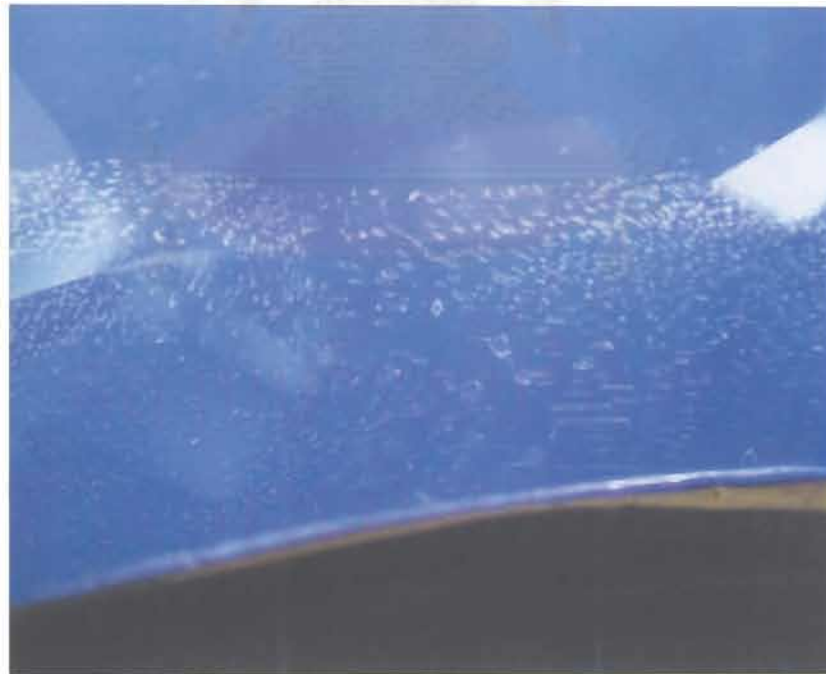
Figure 7.6: The hazy appearance with well-formed fingerprints or healed fractures of the un-heated stone.
