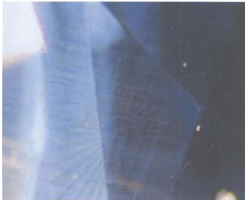
Figure 7.3: Fine long rutile silks associated with very fine particles which make the stone appear bazy typical of un-heated sample.
