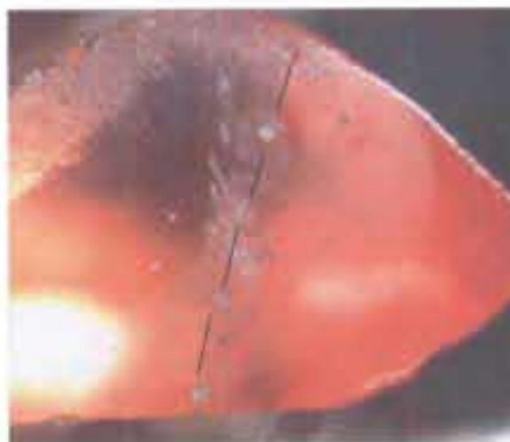
Figure 4.6. A 'classically' heat-treated orange sapphire (KNI) was cut in half and a five-point profile was analyzed across the cut surface using LA-ICP-MS. (Photo by Lomthong, KU)
