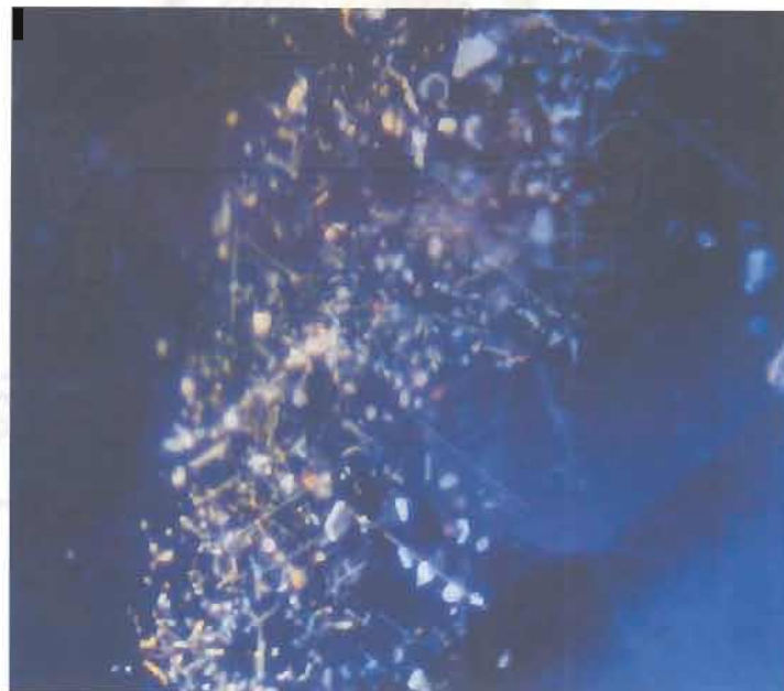
Figure 8.12: This 3.25 ct un-heated Ilakaka sapphire shows hazy appearance. The well-formed continuous long and sharp rutile silks and zones of dust particles are typical of the un-heated stone. (Photos by Somboon, GIT)
