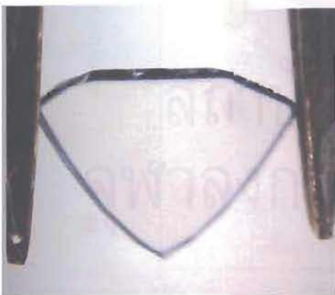
Figure 1.4: An example showing a slice of a classical external Ti diffusion treated sapphire causing the blue coloured rim. Sample size is 4x7 mm (Immersion, Photo by Häger).
