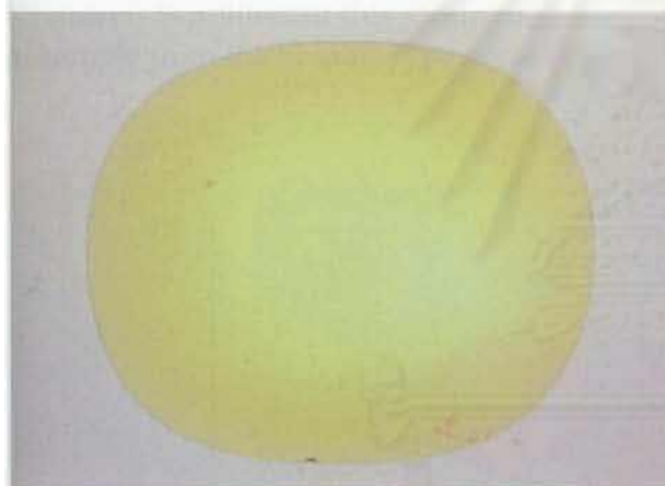
Figure 2: Surface-related colour zones in a yellow sapphire, 10.06 × 11.57 mm. (Immersion, photo by Leelawatanasuk, GIT)
