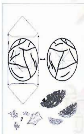
Figure 2c Significant residue (TE5) in this example consisting of coarse and thick film-like structures
