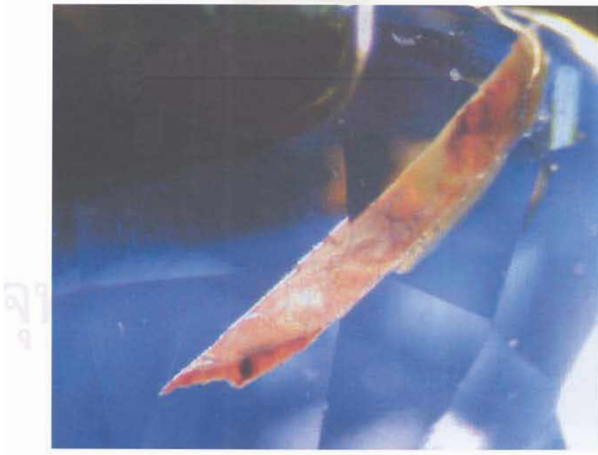
Figure 7.29: The hollow tube filled with dark red impurity is a good indication of un-heated stone .
