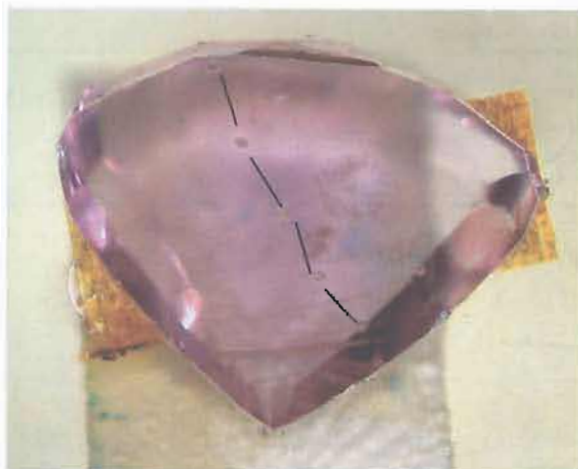
Figure 4.4: An un-treated pink Madagascan sapphire (GITMDP18) was cut in half and a six-point profile was analyzed across the cut surface using LA-ICP-MS. (Photo by Lomthong, KU)
