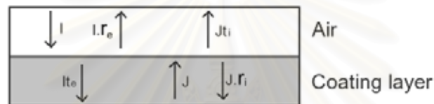
Figure 2.5 Diagram of energy flux at the boundary of air and coating layer [7] .
