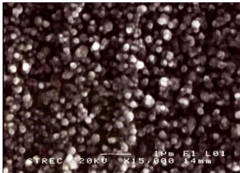
Figure 4.19 : An enlarged (x15,000) picture of the surface of the steel plate after the bombardment of the plasma focus taken by SEM [28].
