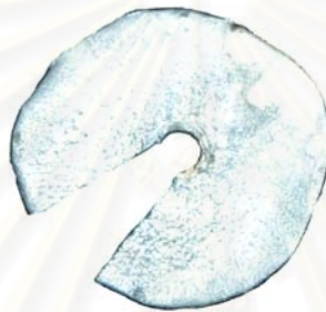
Figure 4.4: A picture showing the damage caused by the bombardment of plasma on the surface of the Aluminum plate which was placed at 2 cm away from the tip of the anode in Argon gas.
