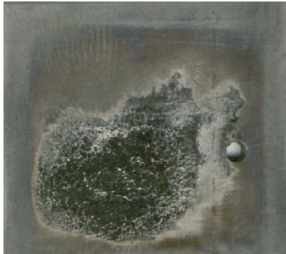
Figure 4.11: A picture showing the surface of the Ti-plate bombarded by ions.
