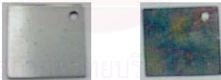
Figure 4.15: A picture of a steel plate taken before and after the firing of the plasma focus [28].
