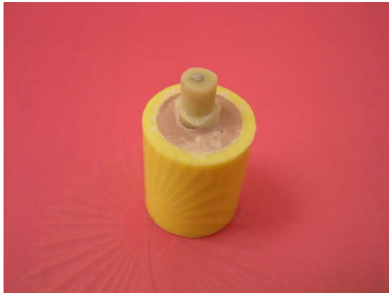
Figure 4 Cylindrical composite core with 4 mm in diameter, perpendicular axial wall, and parallel occlusal surface
