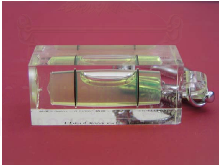
Figure 3 A level for checking occlusal paralleling of the core
