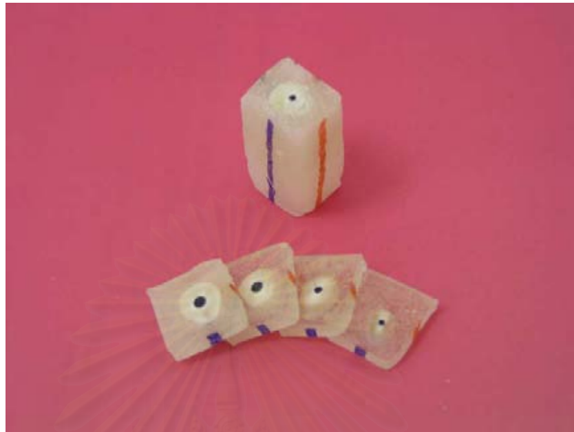
Figure 6 Samples after embedded in clear acrylic resin and cut with Isomet saw
